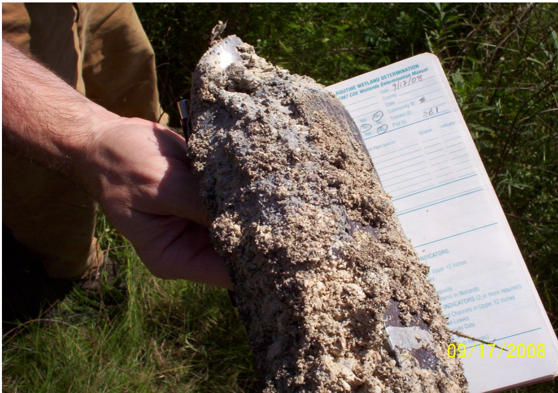
Photo 22. Soil boring sample of SB1 plot from Settling Basin 13.
