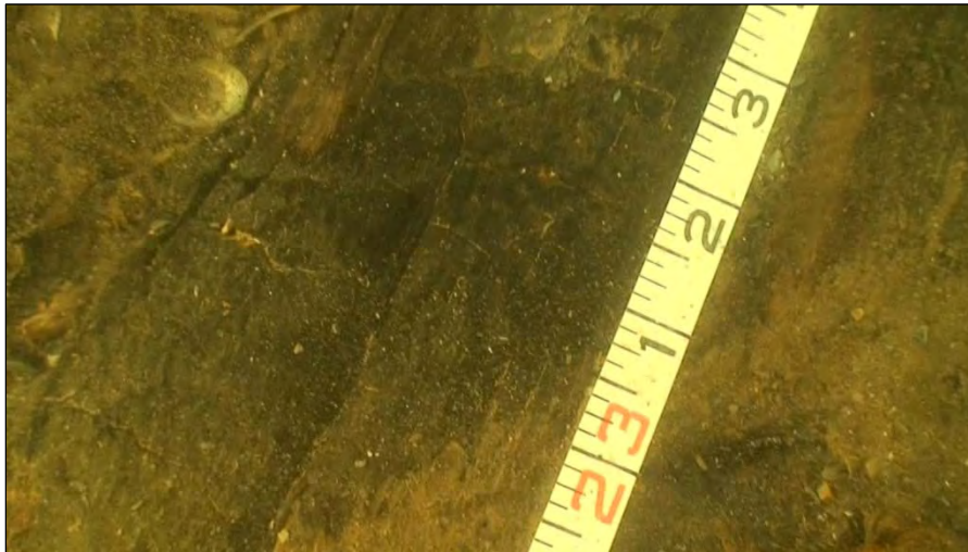
Figure 47: Evidence of charring was visible on the keelson of A2-3 (LCMM Collection).
