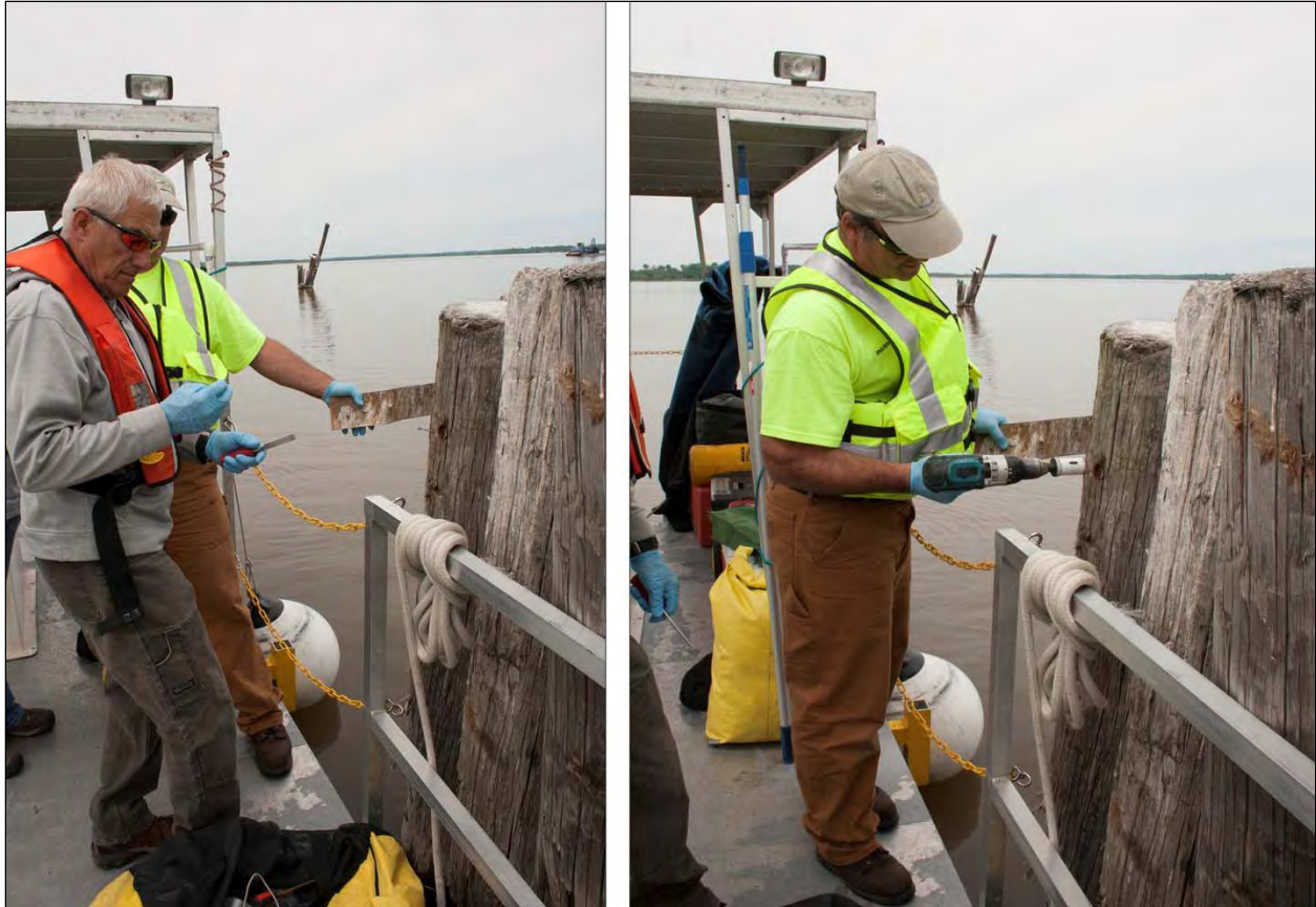
Figure 58: LCMM researchers take wood samples at A7 using chisel (left) and drill (right) (LCMM Collection).
