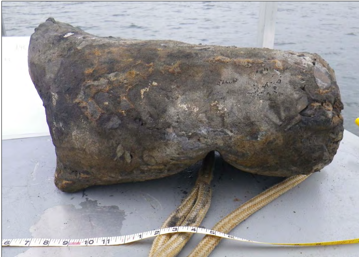
Figure 90: Sample concrete from A45 breakwater (LCMM Collection).
