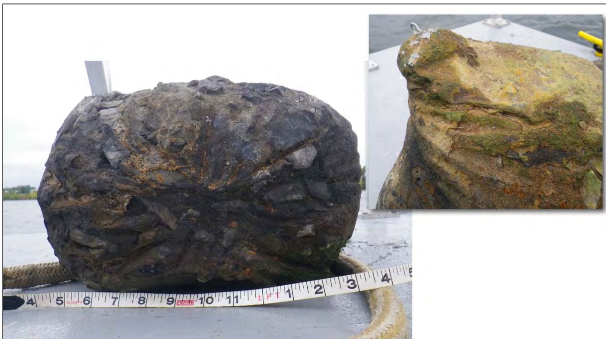
Figure 91: Details from two concrete masses from A45. Note the depressions in the concrete indicating that they were formed by using bags. The inset at right shows burlap-style markings. (LCMM Collection).
