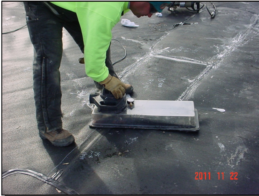
Photograph 7: Extrusion welds were non-destructively tested using the vacuum test method.
