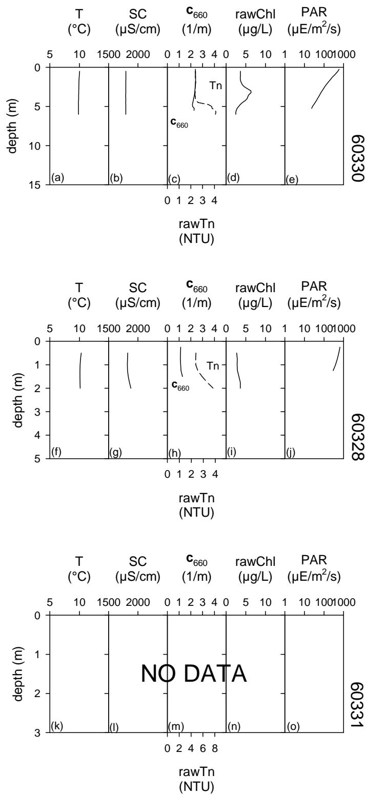
**Figure 28.** Pre-Dredge Monitoring profiles on November 16, 2010 at transect T3 for sites: (a) 60330 temperature (T), (b) 60330 specific conductivity (SC), (c) 60330 turbidity (Tn) and  $c_{660}$ , (d) 60330 chlorophyll a (chl),(e) 60330 photosynthetic active radiation (PAR), (f) 60328 T, (g) 60328 SC, (h) 60328 Tn and  $c_{660}$ , (i) 60328 chl, (j)60328 PAR, (k) 60331 T, (l) 60331 SC, (m) 60331 Tn and  $c_{660}$ , (n) 60331 chl, (o) 60331 PAR.
