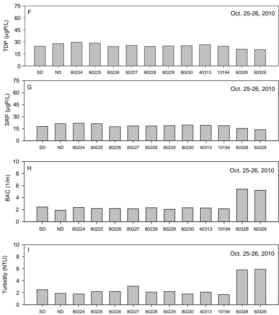
Figure 1. Analytical results for samples collected from 13 locations in Onondaga Lake on October 25 and 26, 2010: (A) chlorophyll *a*, (B) total ammonia, (C) nitrate + nitrite, (D) nitrite, (E) total phosphorus, (F) total dissolved phosphorus, (G) soluble reactive phosphorus, (H) beam attenuation coefficient, and (I) turbidity.
