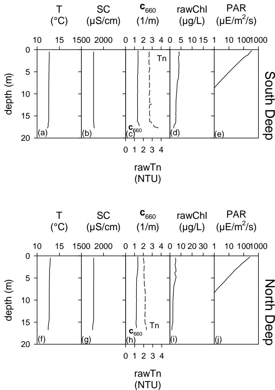
**Figure 10.** Pre-Dredge Monitoring profiles on October 25, 2010 at South Deep and North Deep: (a) South Deep temperature (T), (b) South Deep specific conductivity (SC), (c) South Deep turbidity (Tn) and  $\mathbf{c}_{660}$ , (d) South Deep chlorophyll a (chl), (e) South Deep photosynthetic active radiation (PAR), (f) North Deep T, (g) North Deep SC, (h) North Deep Tn and  $\mathbf{c}_{660}$ , (i) North Deep chl, (j) North Deep PAR.
