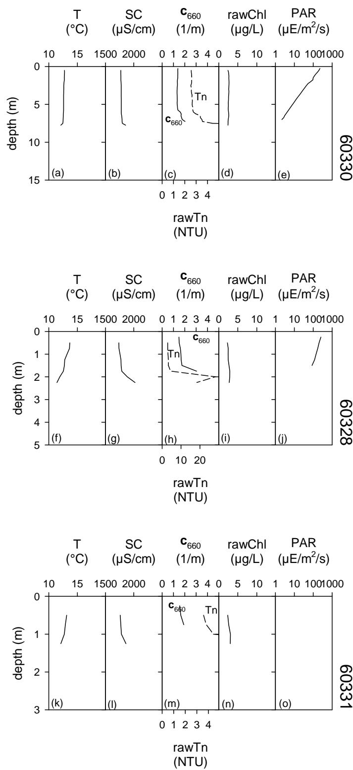
**Figure 8.** Pre-Dredge Monitoring profiles on October 25, 2010 at transect T3 for sites: (a) 60330 temperature (T), (b) 60330 specific conductivity (SC), (c) 60330 turbidity (Tn) and  $c_{660}$ , (d) 60330 chlorophyll a (chl), (e) 60330 photosynthetically active radiation (PAR), (f) 60328 T, (g) 60328 SC, (h) 60328 Tn and  $c_{660}$ , (i) 60328 chl, (j) 60328 PAR, (k) 60331 T, (l) 60331 SC, (m) 60331 Tn and  $c_{660}$ , (n) 60331 chl, (o) 60331 PAR.
