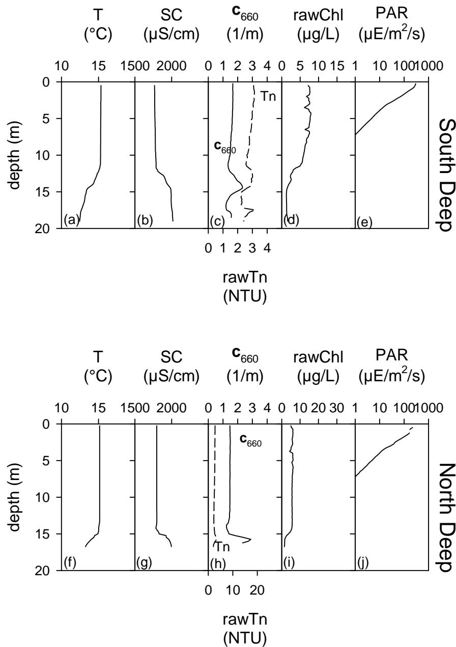
**Figure 5.** Pre-Dredge Monitoring profiles on October 14, 2010 at South Deep and North Deep: (a) South Deep temperature (T), (b) South Deep specific conductivity (SC), (c) South Deep turbidity (Tn) and  $c_{660}$ , (d) South Deep chlorophyll a (chl),(e) South Deep photosynthetic active radiation (PAR), (f) North Deep T, (g) North Deep SC, (h) North Deep Tn and  $c_{660}$ , (i) North Deep chl, (j)North Deep PAR.
