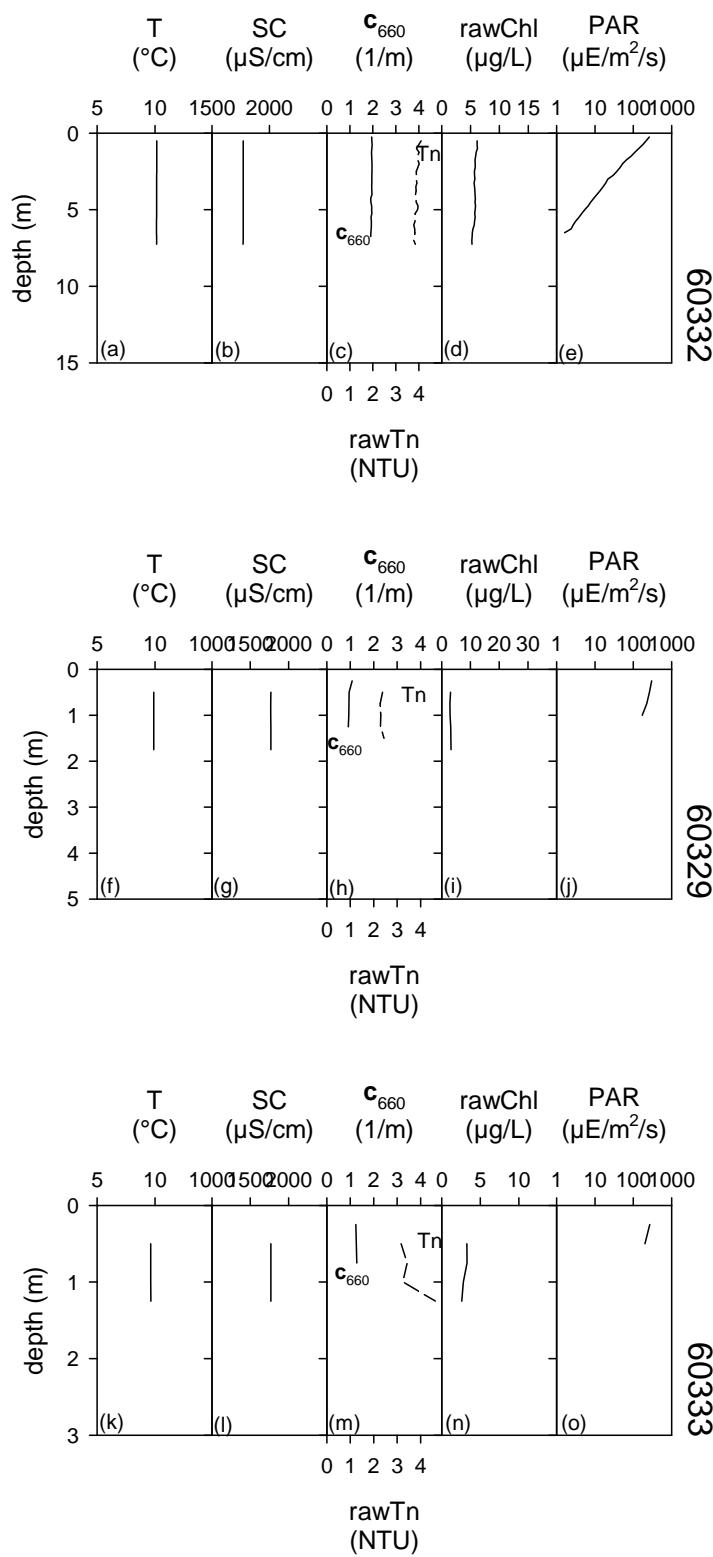
**Figure 24.** Pre-Dredge Monitoring profiles on November 9, 2010 at transect T4 for sites: (a) 60332 temperature (T), (b) 60332 specific conductivity (SC), (c) 60332 turbidity (Tn) and  $c_{660}$ , (d) 60332 chlorophyll a (chl),(e) 60332 photosynthetic active radiation (PAR), (f) 60329 T, (g) 60329 SC, (h) 60329 Tn and  $c_{660}$ , (i) 60329 chl, (j)60329 PAR, (k) 60333 T, (l) 60333 SC, (m) 60333 Tn and  $c_{660}$ , (n) 60333 chl, (o) 60333 PAR.
