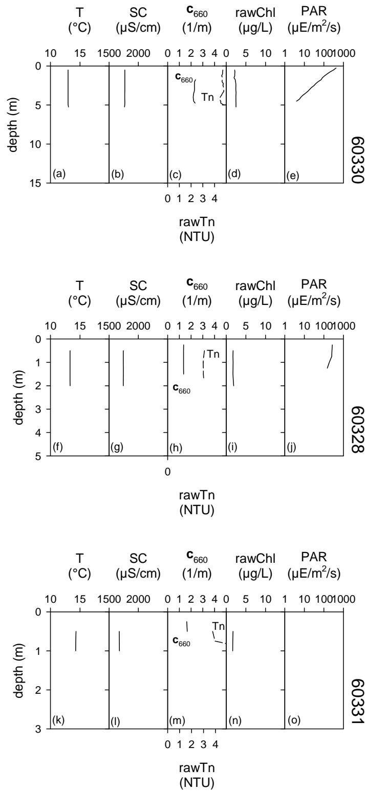
**Figure 13.** Pre-Dredge Monitoring profiles on October 28, 2010 at transect T3 for sites: (a) 60330 temperature (T), (b) 60330 specific conductivity (SC), (c) 60330 turbidity (Tn) and  $c_{660}$ , (d) 60330 chlorophyll a (chl), (e) 60330 photosynthetic active radiation (PAR), (f) 60328 T, (g) 60328 SC, (h) 60328 Tn and  $c_{660}$ , (i) 60328 chl, (j) 60328 PAR, (k) 60331 T, (l) 60331 SC, (m) 60331 Tn and  $c_{660}$ , (n) 60331 chl, (o) 60331 PAR.
