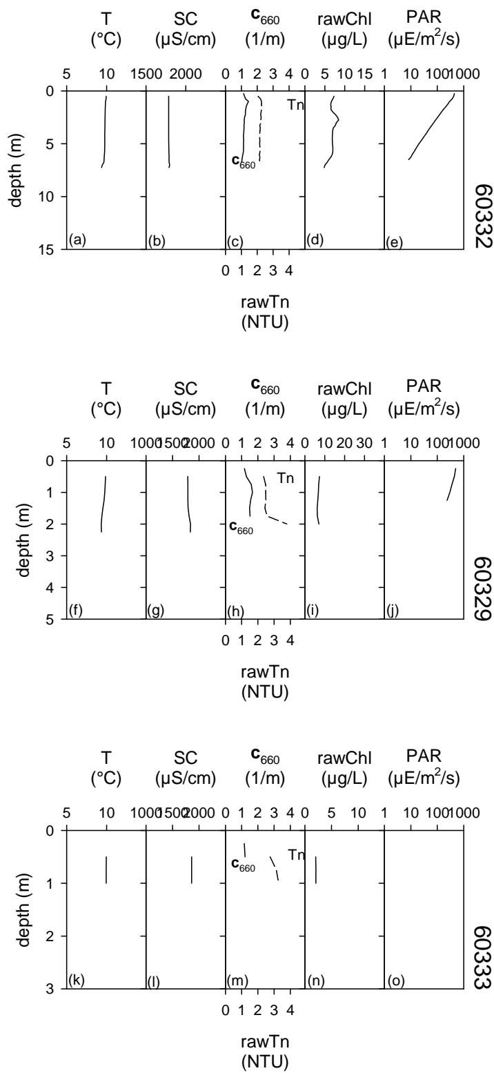
**Figure 29.** Pre-Dredge Monitoring profiles on November 16, 2010 at transect T4 for sites: (a) 60332 temperature (T), (b) 60332 specific conductivity (SC), (c) 60332 turbidity (Tn) and  $c_{660}$ , (d) 60332 chlorophyll a (chl),(e) 60332 photosynthetic active radiation (PAR), (f) 60329 T, (g) 60329 SC, (h) 60329 Tn and  $c_{660}$ , (i) 60329 chl, (j)60329 PAR, (k) 60333 T, (l) 60333 SC, (m) 60333 Tn and  $c_{660}$ , (n) 60333 chl, (o) 60333 PAR.
