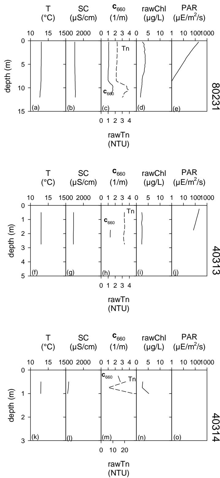
**Figure 11.** Pre-Dredge Monitoring profiles on October 28, 2010 at transect T1 for sites: (a) 80231 temperature (T), (b) 80231 specific conductivity (SC), (c) 80231 turbidity (Tn) and  $c_{660}$ , (d) 80231 chlorophyll a (chl),(e) 80231 photosynthetic active radiation (PAR), (f) 40313 T, (g) 40313 SC, (h) 40313 Tn and  $c_{660}$ , (i) 40313 chl, (j) 40313 PAR, (k) 40314 T, (l) 40314 SC, (m) 40314 Tn and  $c_{660}$ , (n) 40314 chl, (o) 40314 PAR.
