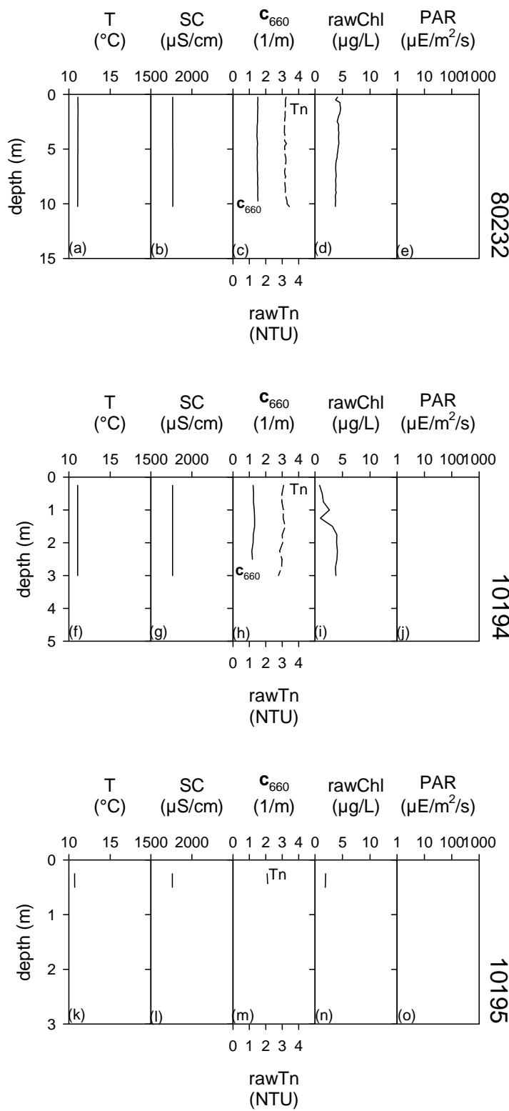
**Figure 17.** Pre-Dredge Monitoring profiles on November 5, 2010 at transect T2 for sites: (a) 80232 temperature (T), (b) 80232 specific conductivity (SC), (c) 80232 turbidity (Tn) and  $c_{660}$ , (d) 80232 chlorophyll a (chl),(e) 80232 photosynthetic active radiation (PAR), (f) 10194 T, (g) 10194 SC, (h) 10194 Tn and  $c_{660}$ , (i) 10194 chl, (j) 10194 PAR, (k) 10195 T, (l) 10195 SC, (m) 10195 Tn and  $c_{660}$ , (n) 10195 chl, (o) 10195 PAR.
