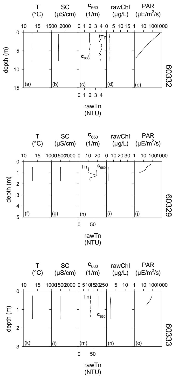
**Figure 14.** Pre-Dredge Monitoring profiles on October 28, 2010 at transect T4 for sites: (a) 60332 temperature (T), (b) 60332 specific conductivity (SC), (c) 60332 turbidity (Tn) and  $c_{660}$ , (d) 60332 chlorophyll a (chl),(e) 60332 photosynthetic active radiation (PAR), (f) 60329 T, (g) 60329 SC, (h) 60329 Tn and  $c_{660}$ , (i) 60329 chl, (j)60329 PAR, (k) 60333 T, (l) 60333 SC, (m) 60333 Tn and  $c_{660}$ , (n) 60333 chl, (o) 60333 PAR.
