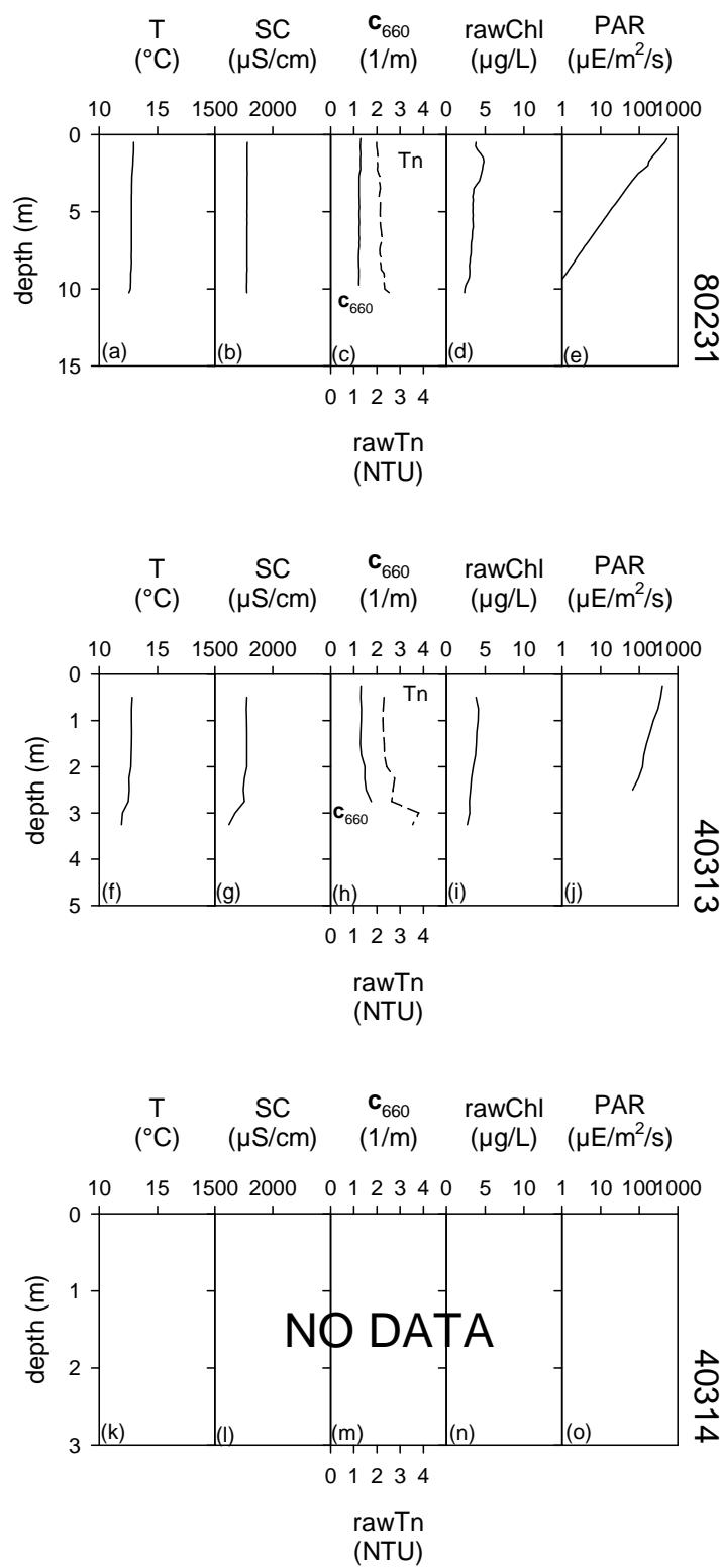
**Figure 6.** Pre-Dredge Monitoring profiles on October 25, 2010 at transect T1 for sites: (a) 80231 temperature (T), (b) 80231 specific conductivity (SC), (c) 80231 turbidity (Tn) and C<sub>660</sub>, (d) 80231 chlorophyll a (chl),(e) 80231 photosynthetic active radiation (PAR), (f) 40313 T, (g) 40313 SC, (h) 40313 Tn and C<sub>660</sub>, (i) 40313 chl, (j) 40313 PAR, (k) 40314 T, (l) 40314 SC, (m) 40314 Tn and C<sub>660</sub>, (n) 40314 chl, (o) 40314 PAR.
