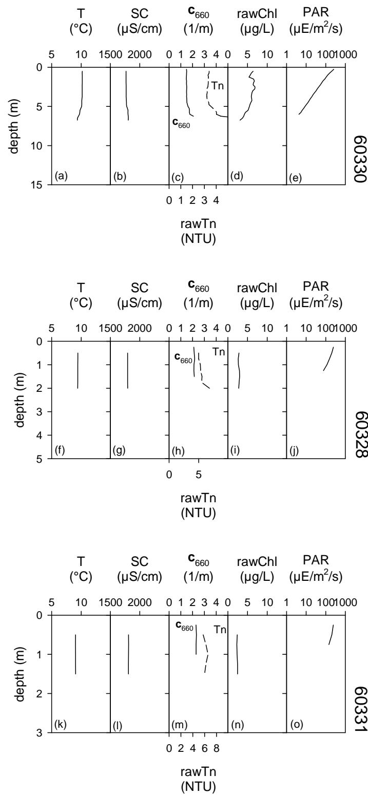
**Figure 23.** Pre-Dredge Monitoring profiles on November 9, 2010 at transect T3 for sites: (a) 60330 temperature (T), (b) 60330 specific conductivity (SC), (c) 60330 turbidity (Tn) and  $c_{660}$ , (d) 60330 chlorophyll a (chl),(e) 60330 photosynthetic active radiation (PAR), (f) 60328 T, (g) 60328 SC, (h) 60328 Tn and  $c_{660}$ , (i) 60328 chl, (j)60328 PAR, (k) 60331 T, (l) 60331 SC, (m) 60331 Tn and  $c_{660}$ , (n) 60331 chl, (o) 60331 PAR.
