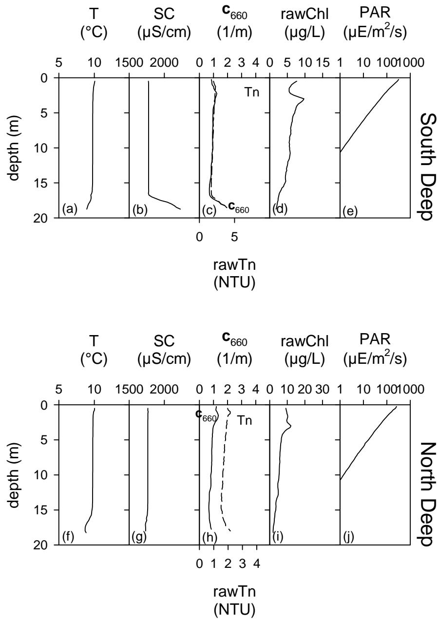
**Figure 30.** Pre-Dredge Monitoring profiles on November 16, 2010 at South Deep and North Deep: (a) South Deep temperature (T), (b) South Deep specific conductivity (SC), (c) South Deep turbidity (Tn) and  $\mathbf{c}_{660}$ , (d) South Deep chlorophyll a (chl), (e) South Deep photosynthetic active radiation (PAR), (f) North Deep T, (g) North Deep SC, (h) North Deep Tn and  $\mathbf{c}_{660}$ , (i) North Deep chl, (j) North Deep PAR.
