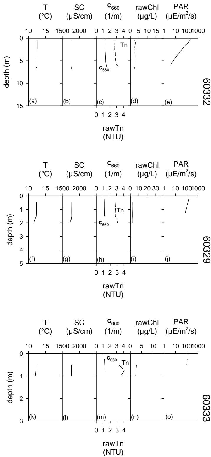
**Figure 9.** Pre-Dredge Monitoring profiles on October 25, 2010 at transect T4 for sites: (a) 60332 temperature (T), (b) 60332 specific conductivity (SC), (c) 60332 turbidity (Tn) and  $c_{660}$ , (d) 60332 chlorophyll a (chl), (e) 60332 photosynthetic active radiation (PAR), (f) 60329 T, (g) 60329 SC, (h) 60329 Tn and  $c_{660}$ , (i) 60329 chl, (j) 60329 PAR, (k) 60333 T, (l) 60333 SC, (m) 60333 Tn and  $c_{660}$ , (n) 60333 chl, (o) 60333 PAR.
