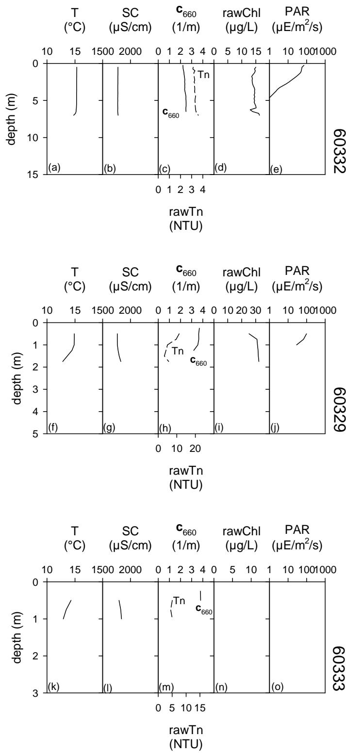
**Figure 4.** Pre-Dredge Monitoring profiles on October 14, 2010 at transect T4 for sites: (a) 60332 temperature (T), (b) 60332 specific conductivity (SC), (c) 60332 turbidity (Tn) and  $c_{660}$ , (d) 60332 chlorophyll a (chl),(e) 60332 photosynthetic active radiation (PAR), (f) 60329 T, (g) 60329 SC, (h) 60329 Tn and  $c_{660}$ , (i) 60329 chl, (j)60329 PAR, (k) 60333 T, (l) 60333 SC, (m) 60333 Tn and  $c_{660}$ , (n) 60333 chl, (o) 60333 PAR.
