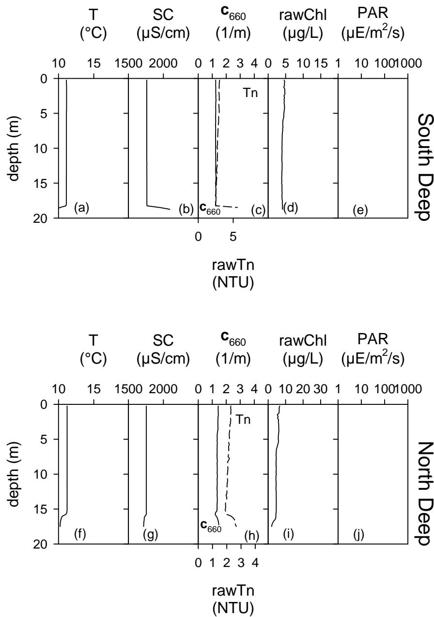
**Figure 20.** Pre-Dredge Monitoring profiles on November 5, 2010 at South Deep and North Deep: (a) South Deep temperature (T), (b) South Deep specific conductivity (SC), (c) South Deep turbidity (Tn) and  $c_{660}$ , (d) South Deep chlorophyll a (chl),(e) South Deep photosynthetic active radiation (PAR), (f) North Deep T, (g) North Deep SC, (h) North Deep Tn and  $c_{660}$ , (i) North Deep chl, (j)North Deep PAR.
