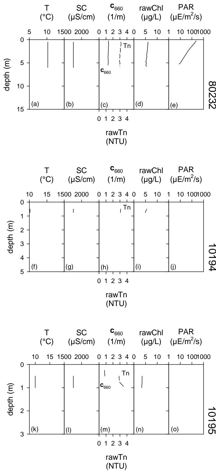
**Figure 22.** Pre-Dredge Monitoring profiles on November 9, 2010 at transect T2 for sites: (a) 80232 temperature (T), (b) 80232 specific conductivity (SC), (c) 80232 turbidity (Tn) and  $c_{660}$ , (d) 80232 chlorophyll a (chl),(e) 80232 photosynthetic active radiation (PAR), (f) 10194 T, (g) 10194 SC, (h) 10194 Tn and  $c_{660}$ , (i) 10194 chl, (j) 10194 PAR, (k) 10195 T, (l) 10195 SC, (m) 10195 Tn and  $c_{660}$ , (n) 10195 chl, (o) 10195 PAR.
