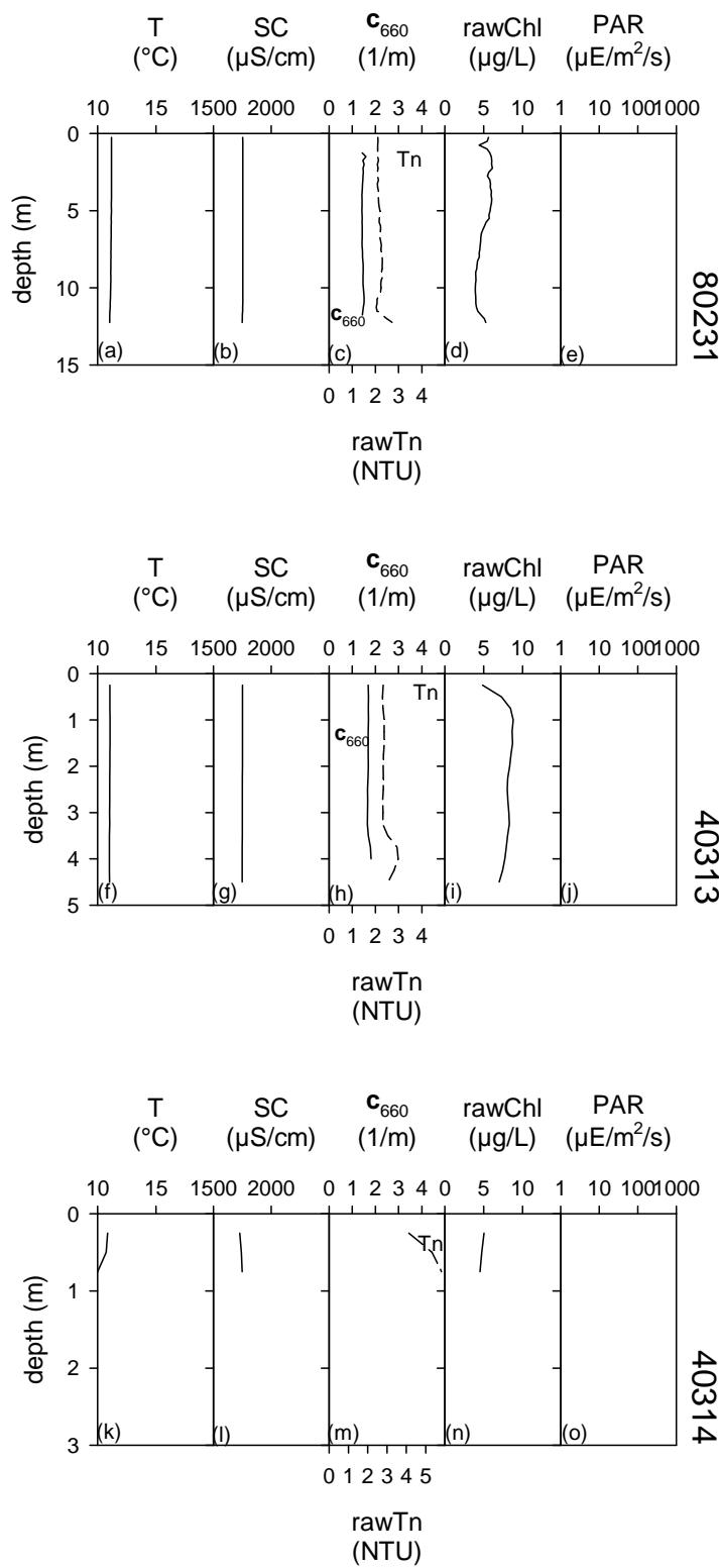
**Figure 16.** Pre-Dredge Monitoring profiles on November 5, 2010 at transect T1 for sites: (a) 80231 temperature (T), (b) 80231 specific conductivity (SC), (c) 80231 turbidity (Tn) and  $c_{660}$ , (d) 80231 chlorophyll a (chl),(e) 80231 photosynthetic active radiation (PAR), (f) 40313 T, (g) 40313 SC, (h) 40313 Tn and  $c_{660}$ , (i) 40313 chl, (j) 40313 PAR, (k) 40314 T, (l) 40314 SC, (m) 40314 Tn and  $c_{660}$ , (n) 40314 chl, (o) 40314 PAR.
