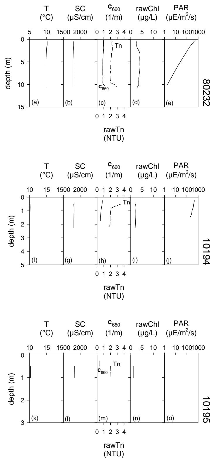
**Figure 27.** Pre-Dredge Monitoring profiles on November 16, 2010 at transect T2 for sites: (a) 80232 temperature (T), (b) 80232 specific conductivity (SC), (c) 80232 turbidity (Tn) and  $c_{660}$ , (d) 80232 chlorophyll a (chl), (e) 80232 photosynthetic active radiation (PAR), (f) 10194 T, (g) 10194 SC, (h) 10194 Tn and  $c_{660}$ , (i) 10194 chl, (j) 10194 PAR, (k) 10195 T, (l) 10195 SC, (m) 10195 Tn and  $c_{660}$ , (n) 10195 chl, (o) 10195 PAR.
