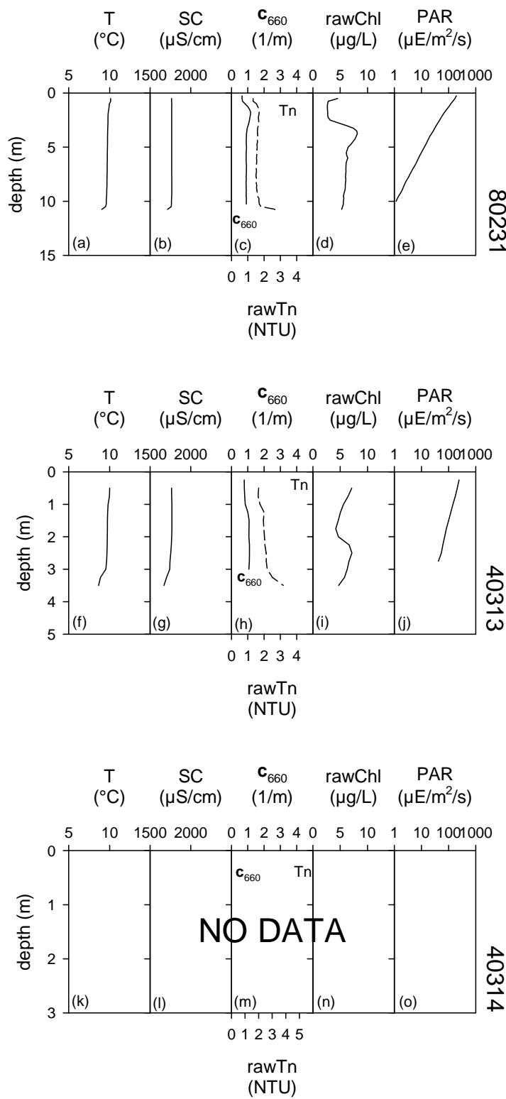
**Figure 26.** Pre-Dredge Monitoring profiles on November 16, 2010 at transect T1 for sites: (a) 80231 temperature (T), (b) 80231 specific conductivity (SC), (c) 80231 turbidity (Tn) and  $c_{660}$ , (d) 80231 chlorophyll a (chl),(e) 80231 photosynthetic active radiation (PAR), (f) 40313 T, (g) 40313 SC, (h) 40313 Tn and  $c_{660}$ , (i) 40313 chl, (j) 40313 PAR, (k) 40314 T, (l) 40314 SC, (m) 40314 Tn and  $c_{660}$ , (n) 40314 chl, (o) 40314 PAR.
