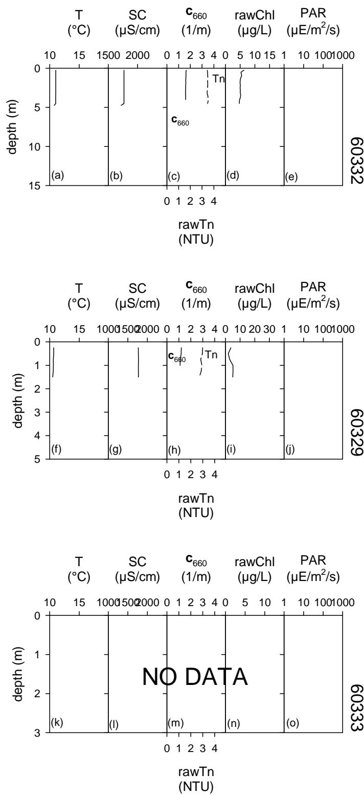
**Figure 19.** Pre-Dredge Monitoring profiles on November 5, 2010 at transect T4 for sites: (a) 60332 temperature (T), (b) 60332 specific conductivity (SC), (c) 60332 turbidity (Tn) and  $\mathbf{c}_{660}$ , (d) 60332 chlorophyll a (chl),(e) 60332 photosynthetic active radiation (PAR), (f) 60329 T, (g) 60329 SC, (h) 60329 Tn and  $\mathbf{c}_{660}$ , (i) 60329 chl, (j)60329 PAR, (k) 60333 T, (l) 60333 SC, (m) 60333 Tn and  $\mathbf{c}_{660}$ , (n) 60333 chl, (o) 60333 PAR.
