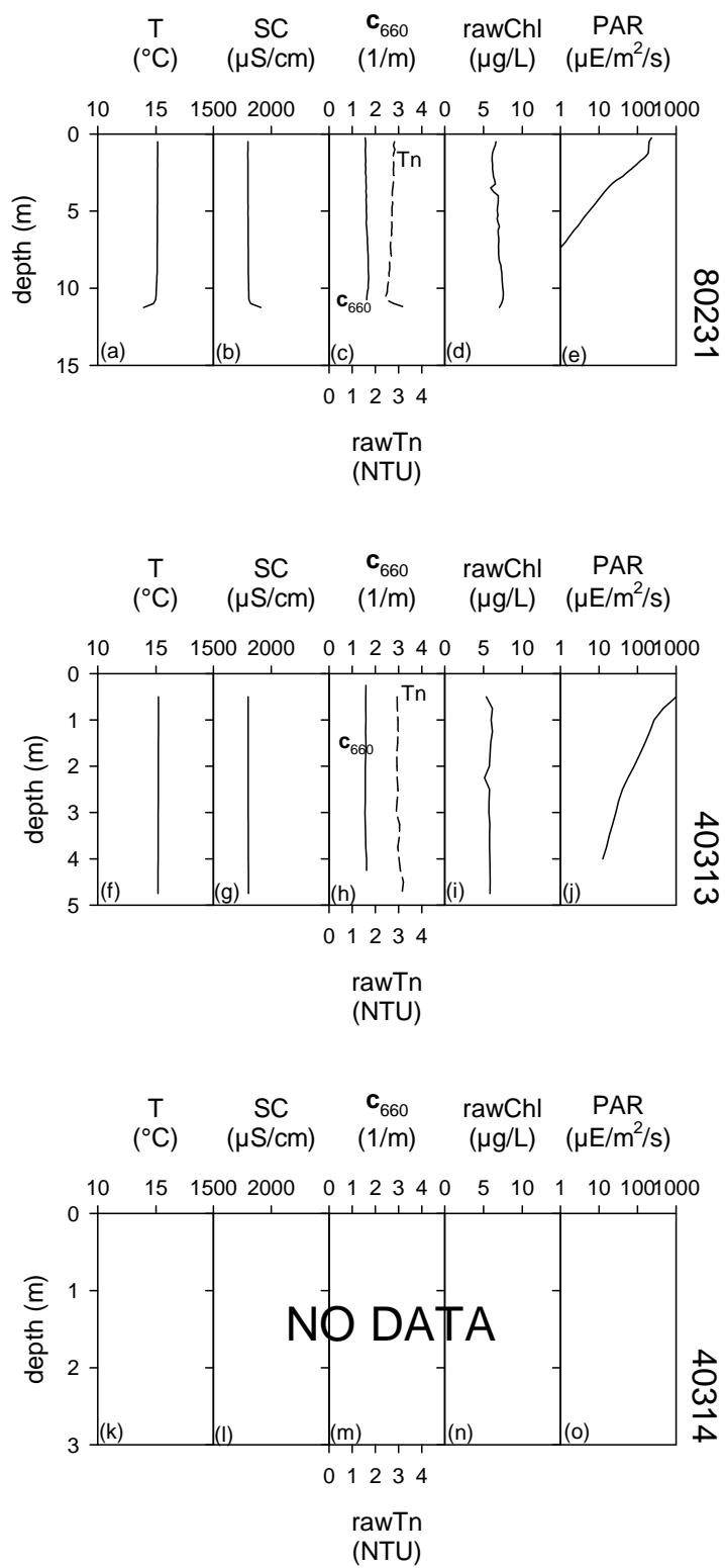
**Figure 1.** Pre-Dredge Monitoring profiles on October 14, 2010 at transect T1 for sites: (a) 80231 temperature (T), (b) 80231 specific conductivity (SC), (c) 80231 turbidity (Tn) and  $c_{660}$ , (d) 80231 chlorophyll a (chl),(e) 80231 photosynthentic active radiation (PAR), (f) 40313 T, (g) 40313 SC, (h) 40313 Tn and  $c_{660}$ , (i) 40313 chl, (j) 40313 PAR, (k) 40314 T, (l) 40314 SC, (m) 40314 Tn and  $c_{660}$ , (n) 40314 chl, (o) 40314 PAR.
