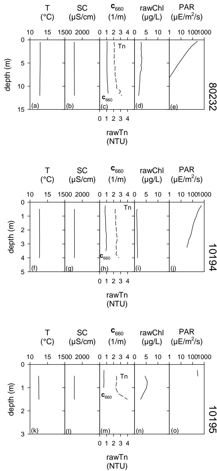
**Figure 12.** Pre-Dredge Monitoring profiles on October 28, 2010 at transect T2 for sites: (a) 80232 temperature (T), (b) 80232 specific conductivity (SC), (c) 80232 turbidity (Tn) and  $c_{660}$ , (d) 80232 chlorophyll a (chl),(e) 80232 photosynthetic active radiation (PAR), (f) 10194 T, (g) 10194 SC, (h) 10194 Tn and  $c_{660}$ , (i) 10194 chl, (j) 10194 PAR, (k) 10195 T, (l) 10195 SC, (m) 10195 Tn and  $c_{660}$ , (n) 10195 chl, (o) 10195 PAR.
