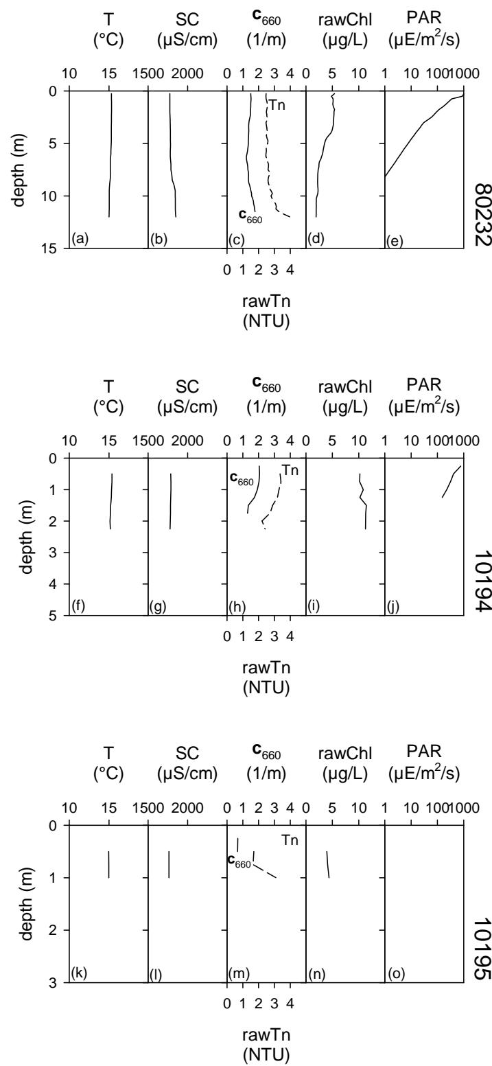
**Figure 2.** Pre-Dredge Monitoring profiles on October 14, 2010 at transect T2 for sites: (a) 80232 temperature (T), (b) 80232 specific conductivity (SC), (c) 80232 turbidity (Tn) and  $c_{660}$ , (d) 80232 chlorophyll a (chl),(e) 80232 photosynthentic active radiation (PAR), (f) 10194 T, (g) 10194 SC, (h) 10194 Tn and  $c_{660}$ , (i) 10194 chl, (j) 10194 PAR, (k) 10195 T, (l) 10195 SC, (m) 10195 Tn and  $c_{660}$ , (n) 10195 chl, (o) 10195 PAR.
