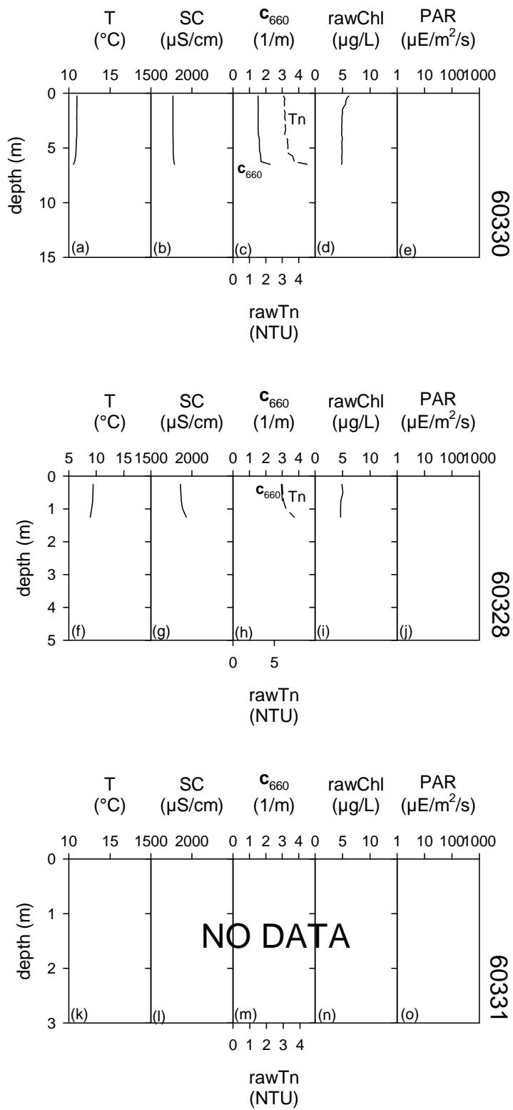
**Figure 18.** Pre-Dredge Monitoring profiles on November 5, 2010 at transect T3 for sites: (a) 60330 temperature (T), (b) 60330 specific conductivity (SC), (c) 60330 turbidity (Tn) and  $c_{660}$ , (d) 60330 chlorophyll a (chl),(e) 60330 photosynthetic active radiation (PAR), (f) 60328 T, (g) 60328 SC, (h) 60328 Tn and  $c_{660}$ , (i) 60328 chl, (j)60328 PAR, (k) 60331 T, (l) 60331 SC, (m) 60331 Tn and  $c_{660}$ , (n) 60331 chl, (o) 60331 PAR.
