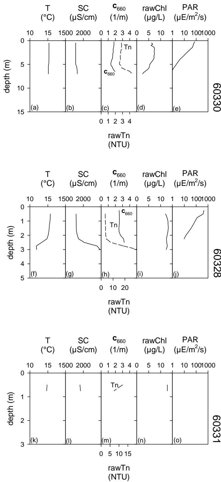
**Figure 3.** Pre-Dredge Monitoring profiles on October 14, 2010 at transect T3 for sites: (a) 60330 temperature (T), (b) 60330 specific conductivity (SC), (c) 60330 turbidity (Tn) and  $c_{660}$ , (d) 60330 chlorophyll a (chl),(e) 60330 photosynthetically active radiation (PAR), (f) 60328 T, (g) 60328 SC, (h) 60328 Tn and  $c_{660}$ , (i) 60328 chl, (j)60328 PAR, (k) 60331 T, (l) 60331 SC, (m) 60331 Tn and  $c_{660}$ , (n) 60331 chl, (o) 60331 PAR.
