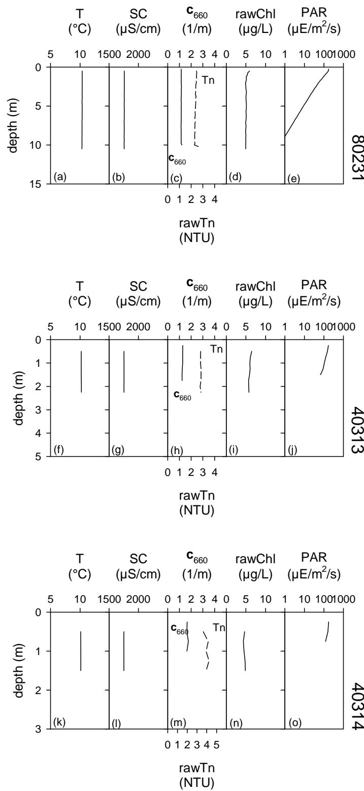
**Figure 21.** Pre-Dredge Monitoring profiles on November 9, 2010 at transect T1 for sites: (a) 80231 temperature (T), (b) 80231 specific conductivity (SC), (c) 80231 turbidity (Tn) and  $c_{660}$ , (d) 80231 chlorophyll a (chl), (e) 80231 photosynthetic active radiation (PAR), (f) 40313 T, (g) 40313 SC, (h) 40313 Tn and  $c_{660}$ , (i) 40313 chl, (j) 40313 PAR, (k) 40314 T, (l) 40314 SC, (m) 40314 Tn and  $c_{660}$ , (n) 40314 chl, (o) 40314 PAR.
