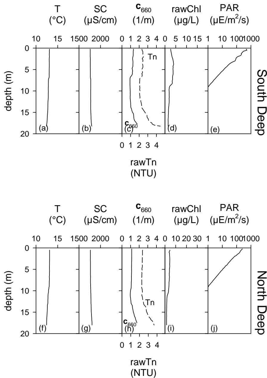
**Figure 15.** Pre-Dredge Monitoring profiles on October 28, 2010 at South Deep and North Deep: (a) South Deep temperature (T), (b) South Deep specific conductivity (SC), (c) South Deep turbidity (Tn) and  $c_{660}$ , (d) South Deep chlorophyll a (chl), (e) South Deep photosynthetic active radiation (PAR), (f) North Deep T, (g) North Deep SC, (h) North Deep Tn and  $c_{660}$ , (i) North Deep chl, (j) North Deep PAR.
