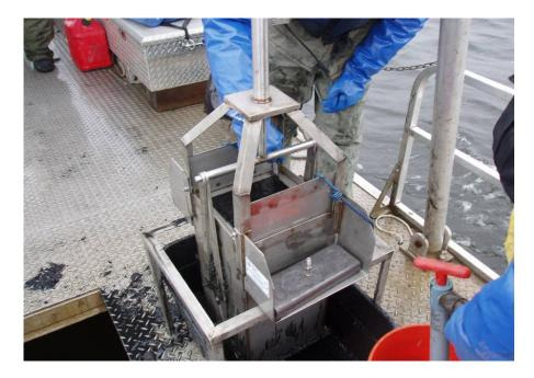
**Collection Step 7:** A hand operated bilge pump was used to slowly remove the excess water above the water-sediment interface, leaving approximately 3 to 4 inches of water above the sediment and with out visibly disturbing the to of the sediment. After water is removed, further observations such as color, odor, and material are noted in the field book.
