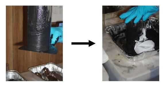
**Processing Step 9**: The sample was then moved to a clean aluminum pan that was used to homogenize the sediment within a particular sampling interval from each of the three tubes collected from a single sampling location. For instance, there was one pan designated for the 0 to 2 cm interval, one for the 2 to 4 cm interval, etc. Each pan held three sample intervals mixed together as a means to collect a representative sample from each sampling interval at each location.
