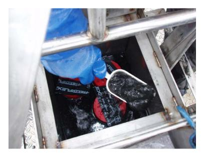
**Cllection Step 12:** The tubes were then carefully removed, vertically, from the box corer. One crew member reached into the box corer pulling the tubes up while reaching beneath the tube as it surfaced and placing a cap under the bottom of the tube.
