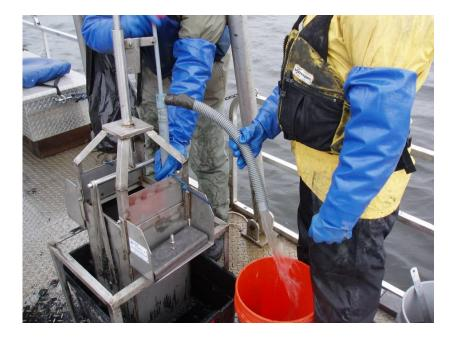
**Collection Step 8:** Pre-cut 12-inch (length) by 3-inch (diameter) Lexan tubes were then capped on one end, labeled, and a small slit was put through the cap in order to allow air to release from the tube as it was pushed into the sediment within the box corer.
