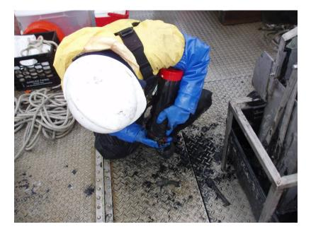
**Collection Step 15:** Once all three tubes were capped and removed from the box corer, excess sediment was wiped from the outside of the tube and caps, and the caps were secured onto the tubes with pipe tape. Tubes were labeled and stored in a vertical position at all times and kept on ice until brought to shore for sample processing.
