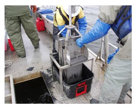
**Collection Step 5:** Approximately 8 to 15 inches (depending on the sample) of water was present above the sediment, filling the box core to the top. Observations such as water color, presence of wax-like film, are noted at this time in the field book.
