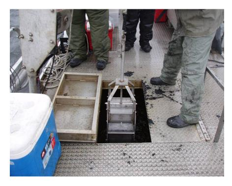
**Collection Step 3:** Once the box core was brought to the boat deck, it was placed into a holding rack with a collection bucket beneath to collect excess sediment.
