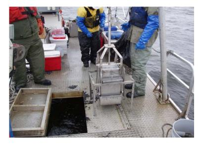
**Collection Step 2:** The box corer was slowly lowered through the center of the boat, using a winch and cathead, until the corer reached the sediment. A lessening of tension in the winch cable was observed at every location when the corer reached the sediment. The box corer with the sediment sample was then slowly raised causing the sample jaws to close.
