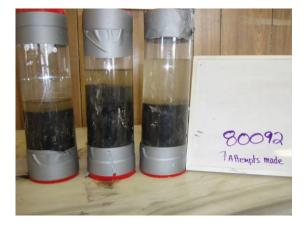
**Processing Step 2**: Without removing surface sediment, liquid was slowly siphoned away from the sediment using a sanitized, plastic syringe that was decontaminated inbetween core sections.
