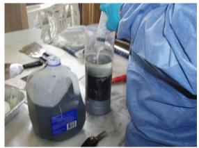
**Processing Step 3**: Once the liquid was decanted, the bottom cap was removed using a retractable blade utility knife. A PVC plug was then inserted into the base of the tube to allow the tube and its contents to be placed on a pedestal. The tube was slowly pushed down on the pedestal forcing the sediment to be pushed up to extract the necessary intervals.
