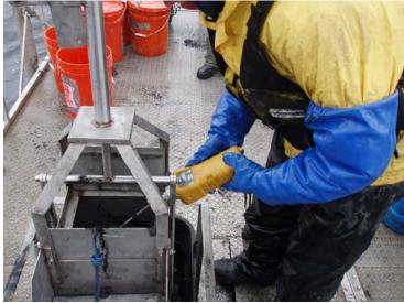
**Collection Step 17:** Finally, a HANNA 9025, with temperature and pH probes was pushed into the remaining sediment for corresponding readings. Readings were recorded in the field book as well as in the electronic database.
