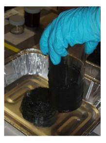
**Processing Step 10**: Once sample from all three tubes were processed, the sediment was homogenized using plastic spoons or nitrile gloved hands. Finally, the sediment was weighed and then placed into the appropriate jars for laboratory analysis. After all sample jars were filled, any remaining sediment was composited into a 1-pint sample jar and labeled for Geotechnical analysis for 0 to 15 cm.
