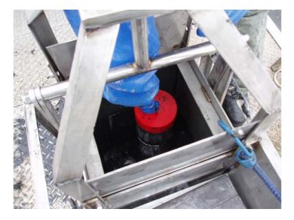
**Collection Step 10:** Once all three tubes were inserted into the box corer as described above, a piece of pipe tape was placed over the slit on each of the caps, thus creating a suction allowing the tube with sediment to be lifted vertical from the box corer losing minimum sediment from the bottom.
