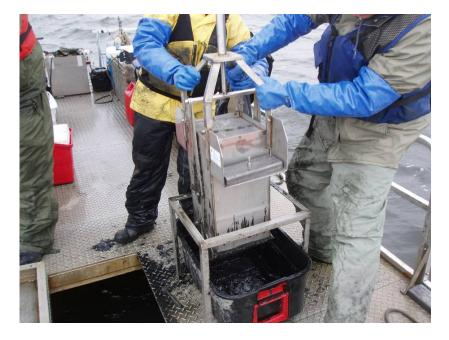
**Collection Step 4:** The top of the box corer opens by two overlapping flaps, which allow for a narrow space where samples are collected carefully through the top.
