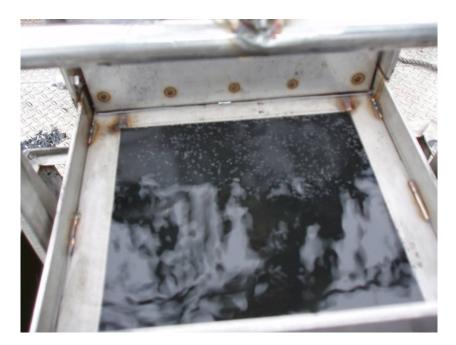
**Collection Step 6:** An 18-inch stainless steel ruler was used to measure the depth of the water above the water-sediment interface, which allowed the thickness of sediment recovery to be estimated. (The crew was able to insert the ruler slowly into the box corer and feel the difference in resistance when the water-sediment interface was reached.)
