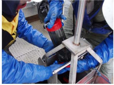
**Collection Step 14:** The bottom cap was secured to the Lexan tube, while keeping the tube in a vertical position and minimizing any sediment loss.
