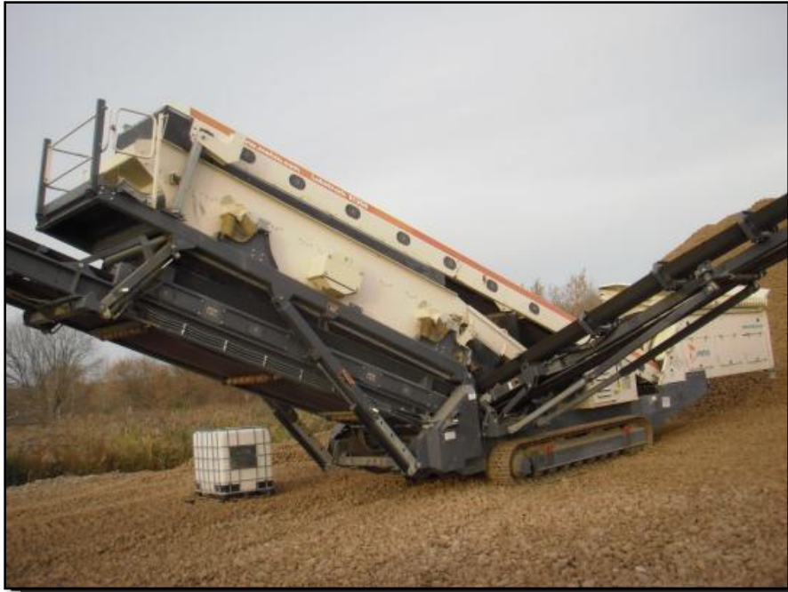
Photograph 37: On 2 November 2011 a screening unit fitted with a wash bar was mobilized to the site to process the gravel on site.
