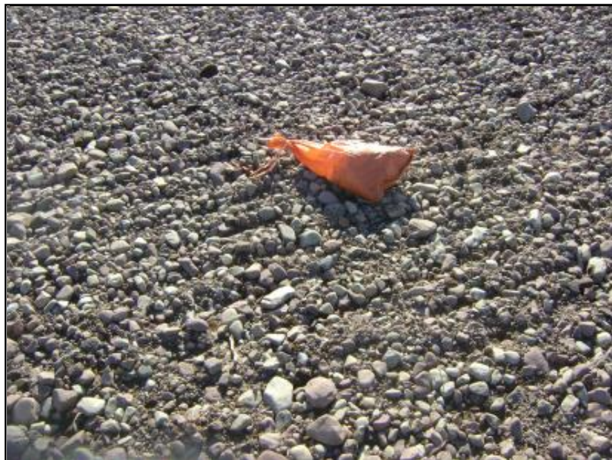
Photographs 35 and 36: Areas of excessive fines were noted in the gravel drainage layer. These areas were marked out using orange sand bags.
