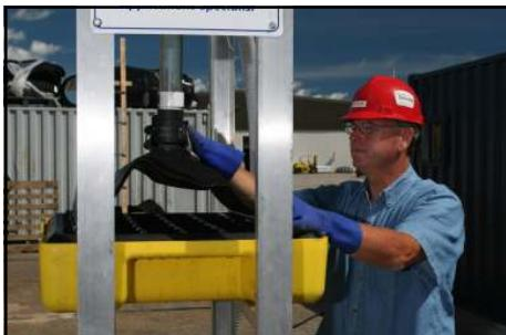
Sample quantity varies depending on slurry type and percent of solids of slurry.
