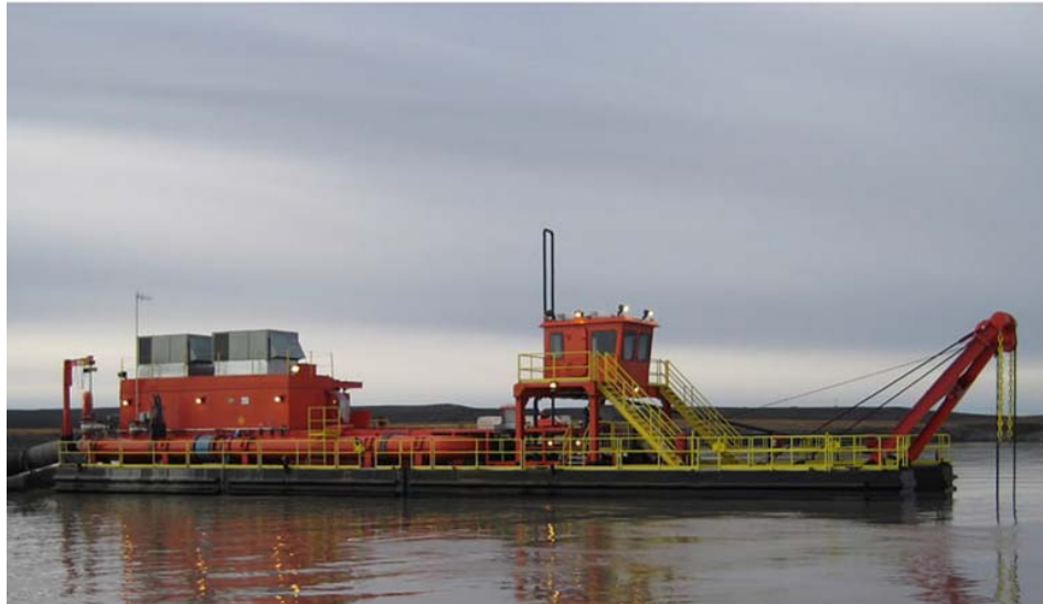
Figure 2. Dredging Supply Company 14-inch-diameter Dredge “Shark”
