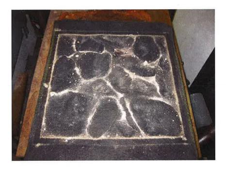
Figure 3. "Prints" of stone on top surface of the nonwoven geotextile after the completion of test.
