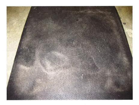
Figure 5. Deformed top surface of the geomembrane (no punctures)
