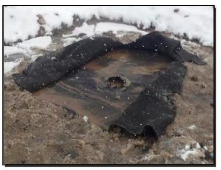
Photograph 31: Abandonment of inclinometer SI-G1 and removal of the associated boot left an approximately 6-in diameter hole within the geomembrane.
