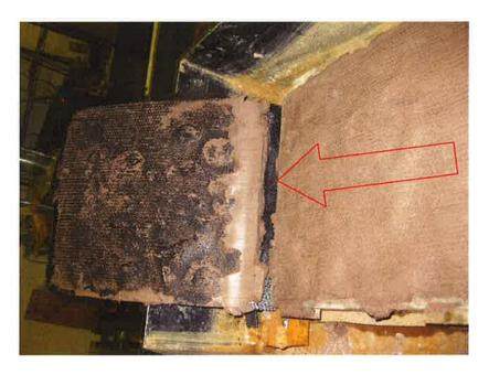
Figure 4. Deformed sgeomembrane and clay surfaces at the completion of Test #1C at 3500 psf.
