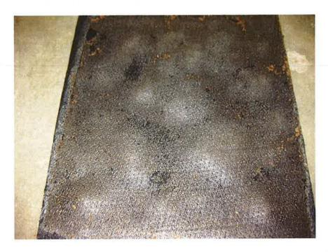
Figure 6. Deformed bottom surface of the geomembrane (no punctures)
