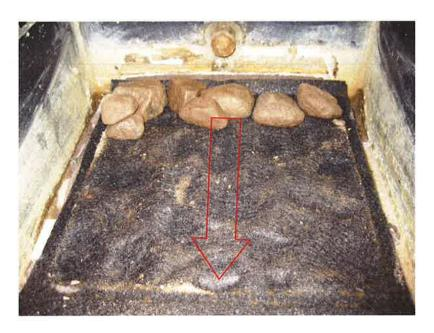
Figure 1. Drainge gravel and 24 oz nonwoven geotextile at the completion of Test #1C (3500 psf)
