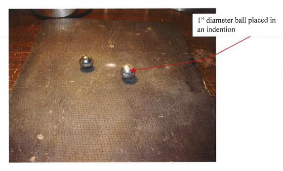
Figure 8. View of indentions on the deformed top surface of the geomembrane
