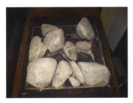
Figure 2. View of stone in contact with the nonwoven geotextile after the completion of test.
