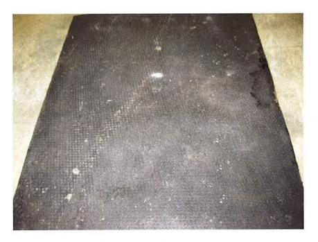
Figure 5. Deformed top surface of the geomembrane (no punctures)
