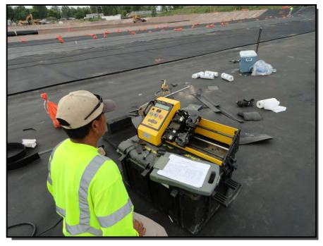
Photograph 14: Calibrated tensiometers were used to conduct field testing of trial welds and destructive samples.
