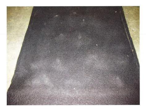
Figure 4. Deformed bottom surface of the geotextile.
