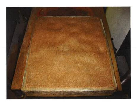
Figure 7. Deformed top surface of subgrade soil
