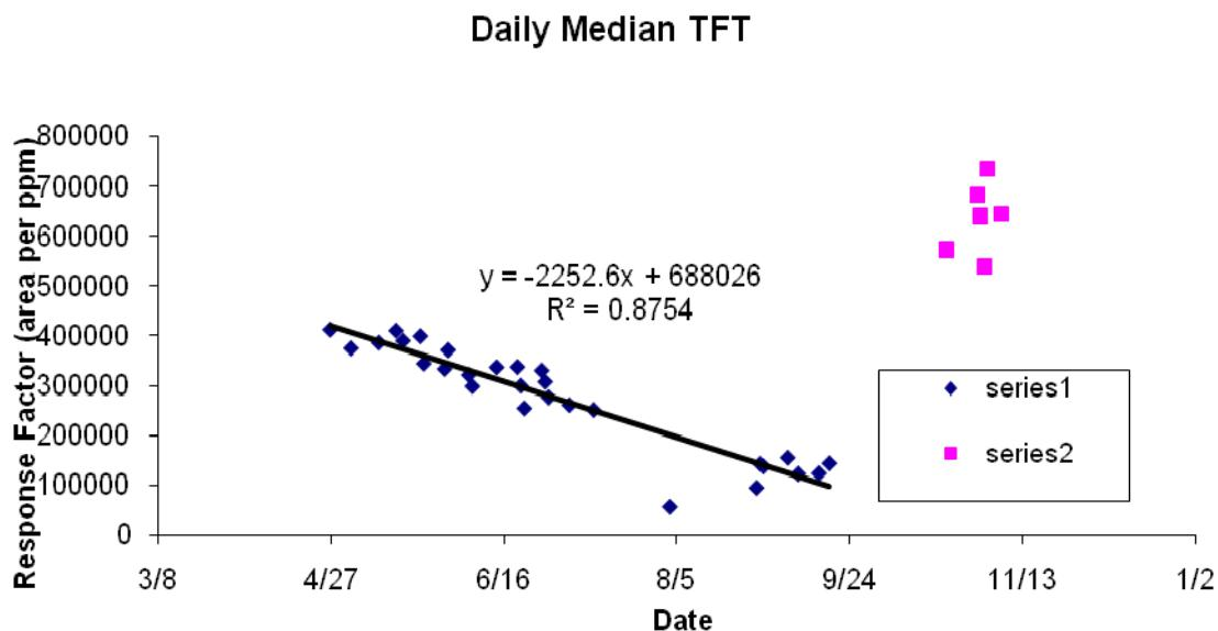
**Figure 1.1.1 Median TFT Response with Time**
