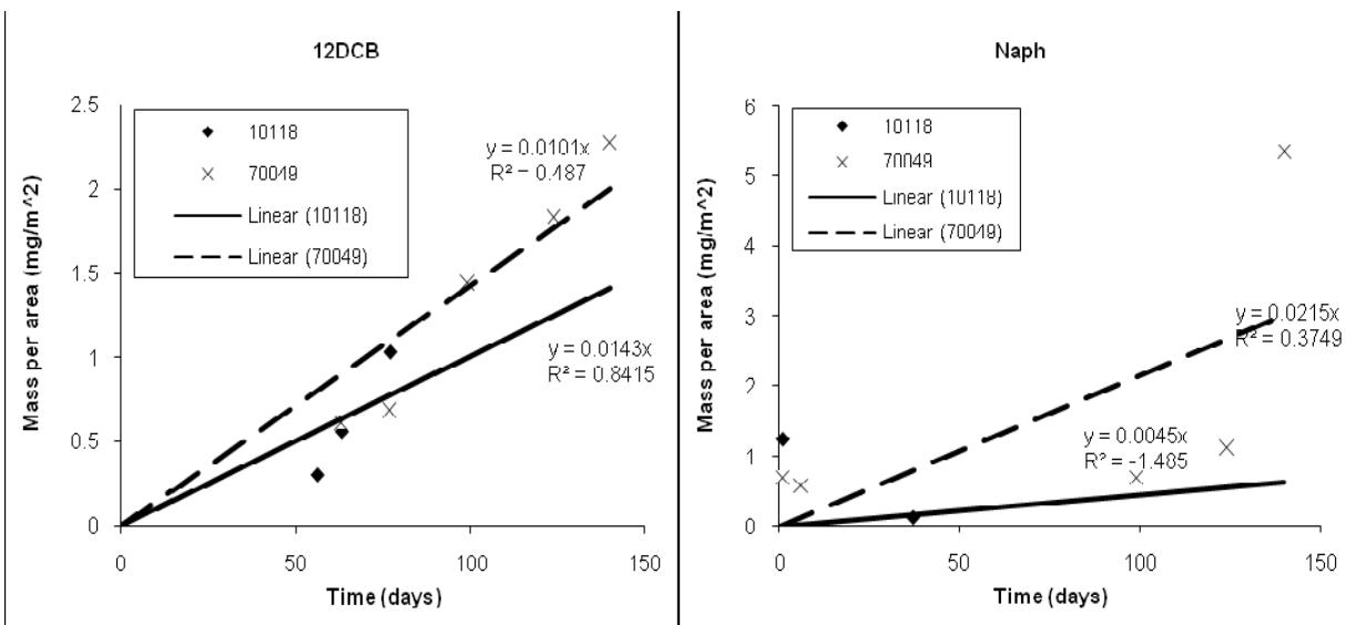
Sediment from locations 10116 and 70048 were subject to gas flow and contaminant flux was measured. Two calibrations were required as the instrument configuration changed during the course of the experiment.
