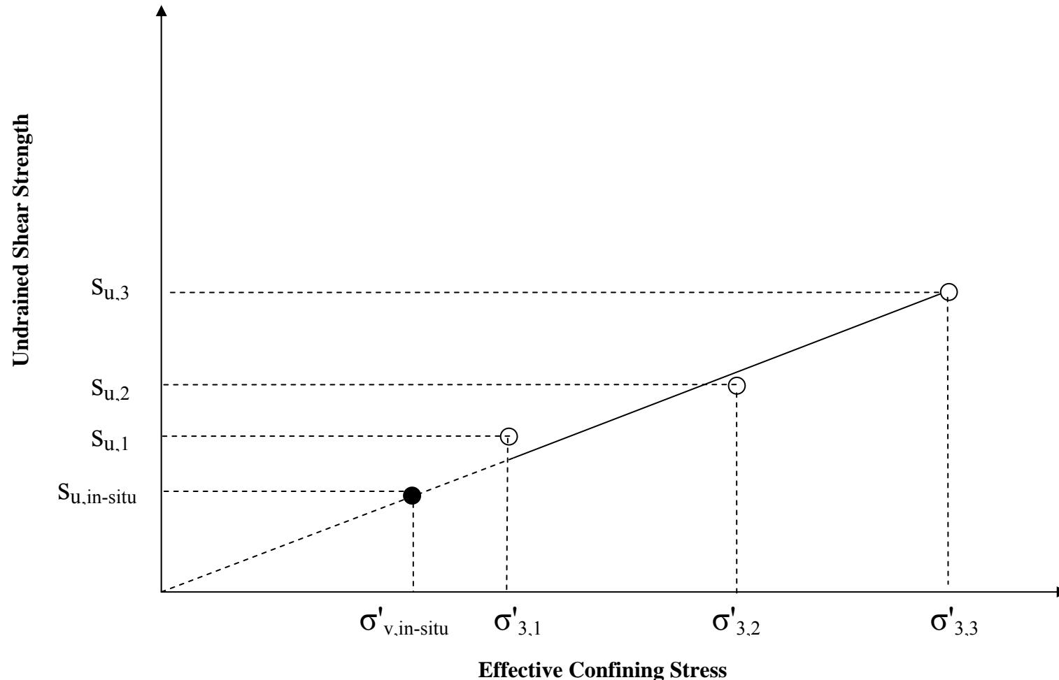
Figure 22. Obtaining  $S_u$  corresponding to the in-situ vertical stress from CU tests (Approach 2).
