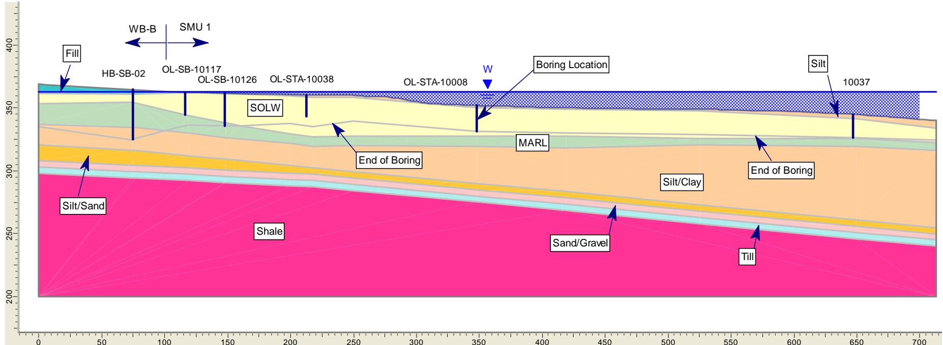
Figure 7. Geometry of cross section 5
