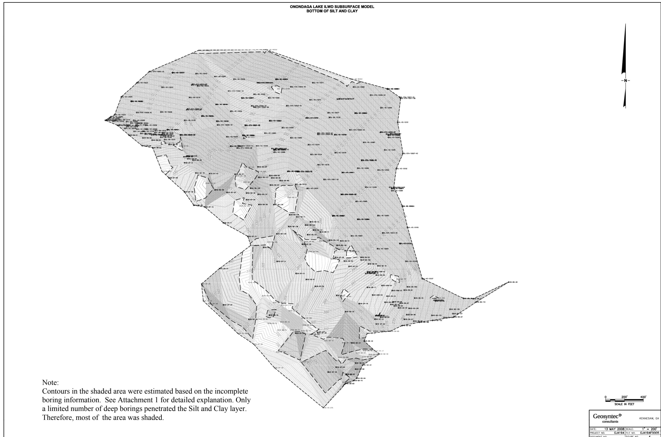
Figure 1-5. Contours of bottom of Silt and Clay
