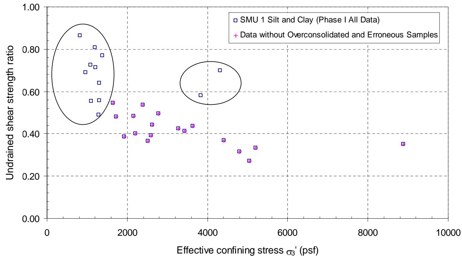
Figure 26. Example of removed samples from CU tests
