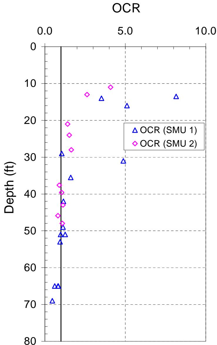
Figure 20. Profile of overconsolidation ratio
