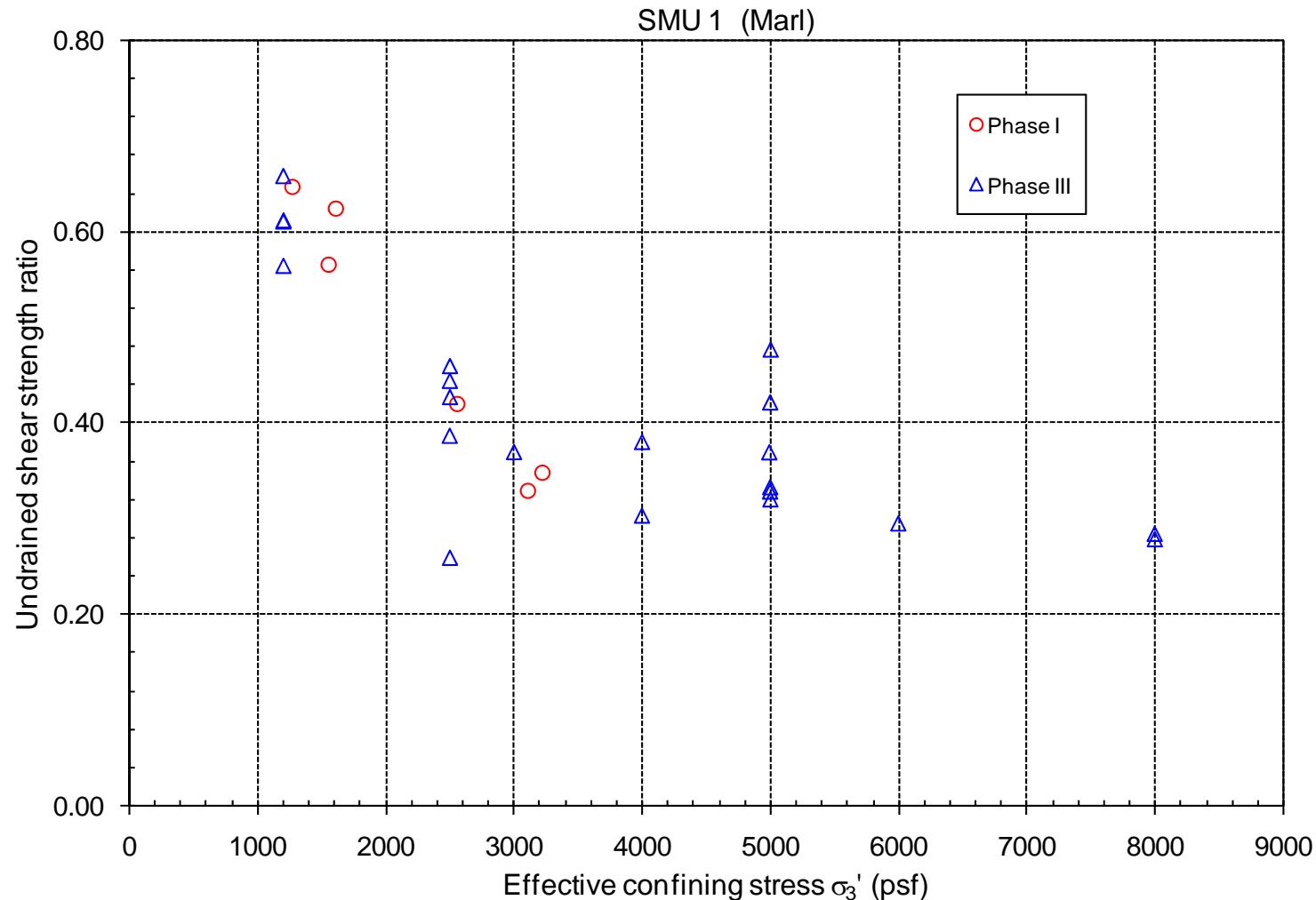
Figure 24. Undrained shear strength ratio for Marl from CU tests
