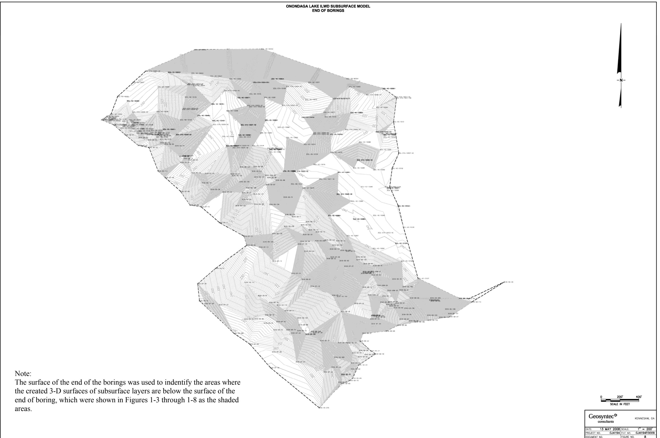
Figure 1-9. Contours of End of Boring
