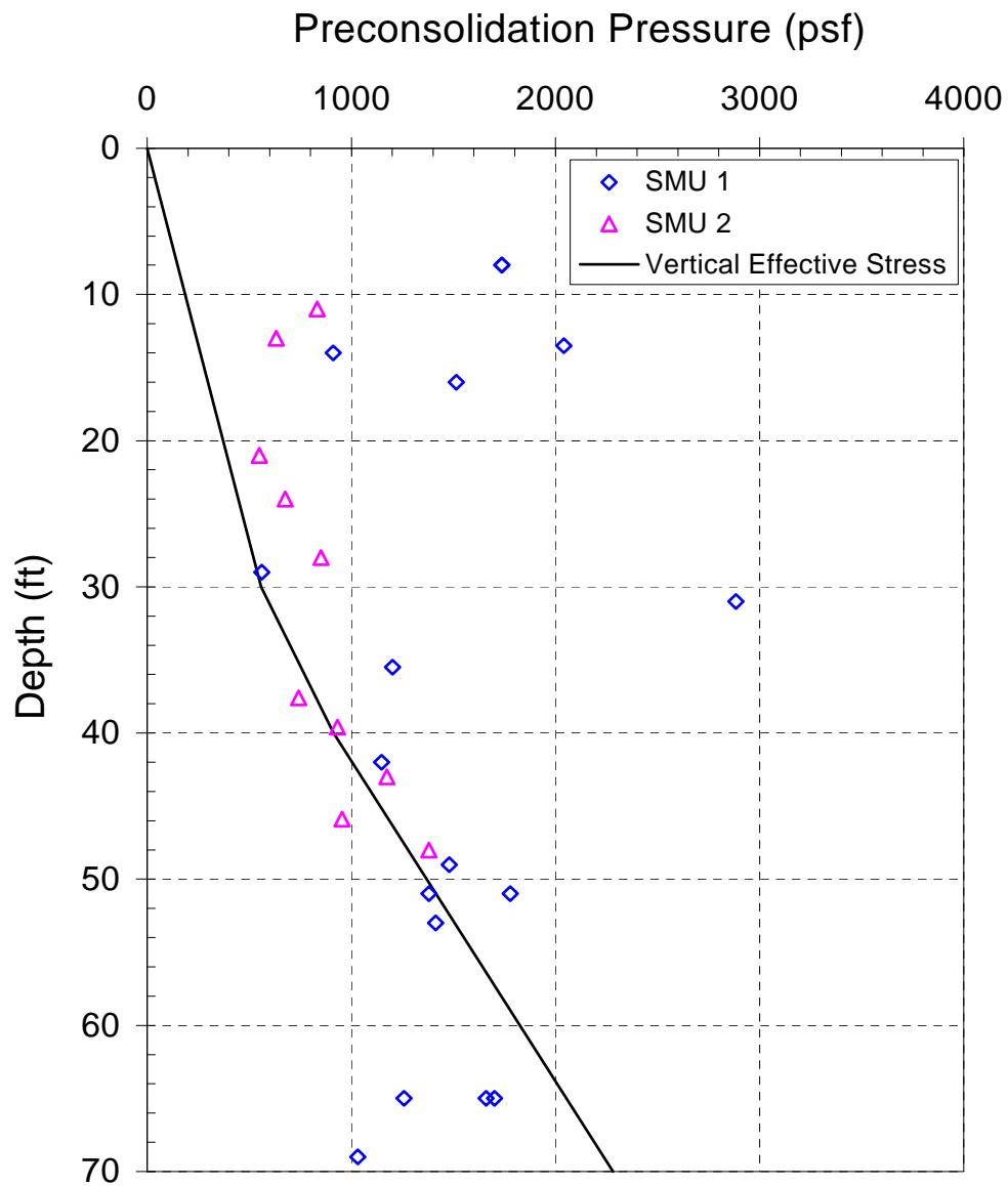
Figure 18. Profile of preconsolidation pressure
