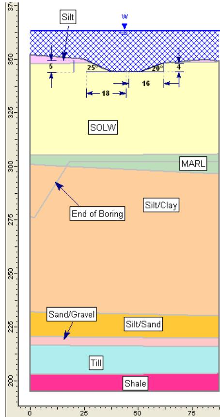
Figure 10. Geometry of cross section 8
