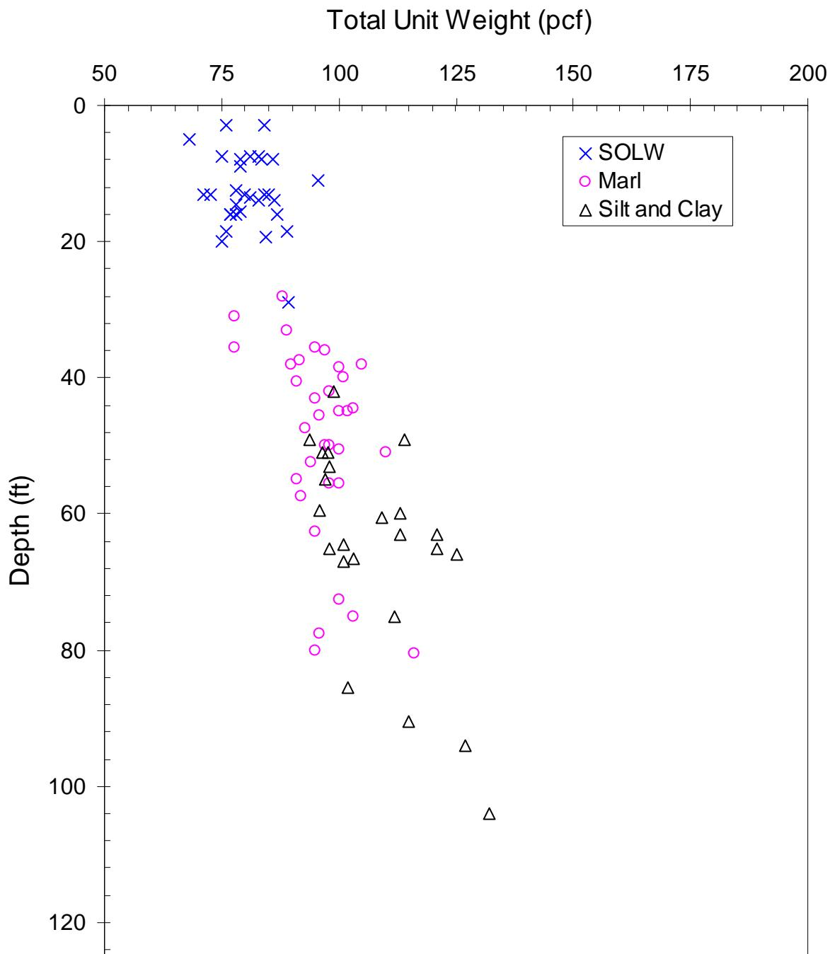
Figure 17. Plot of total unit weight versus depth
