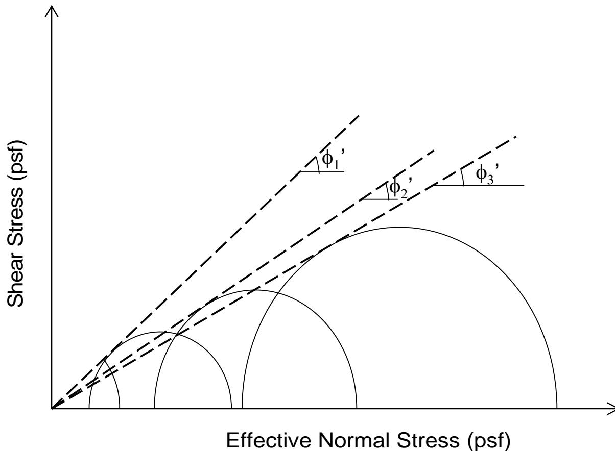
Figure 29. Obtaining effective stress friction angle using effective stress Mohr circles from CU tests
