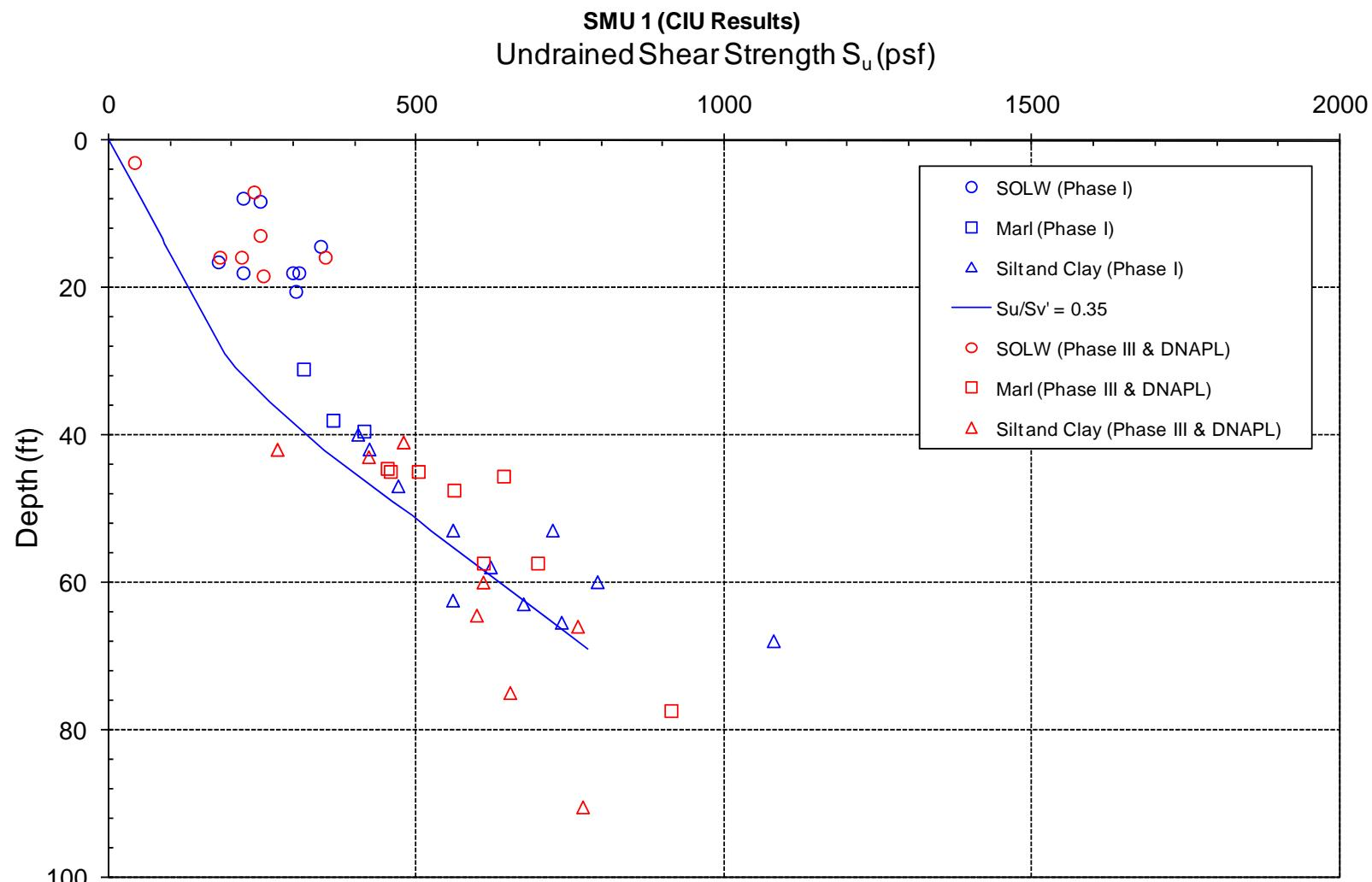
Figure 27. Interpreted undrained shear strength from CU tests
