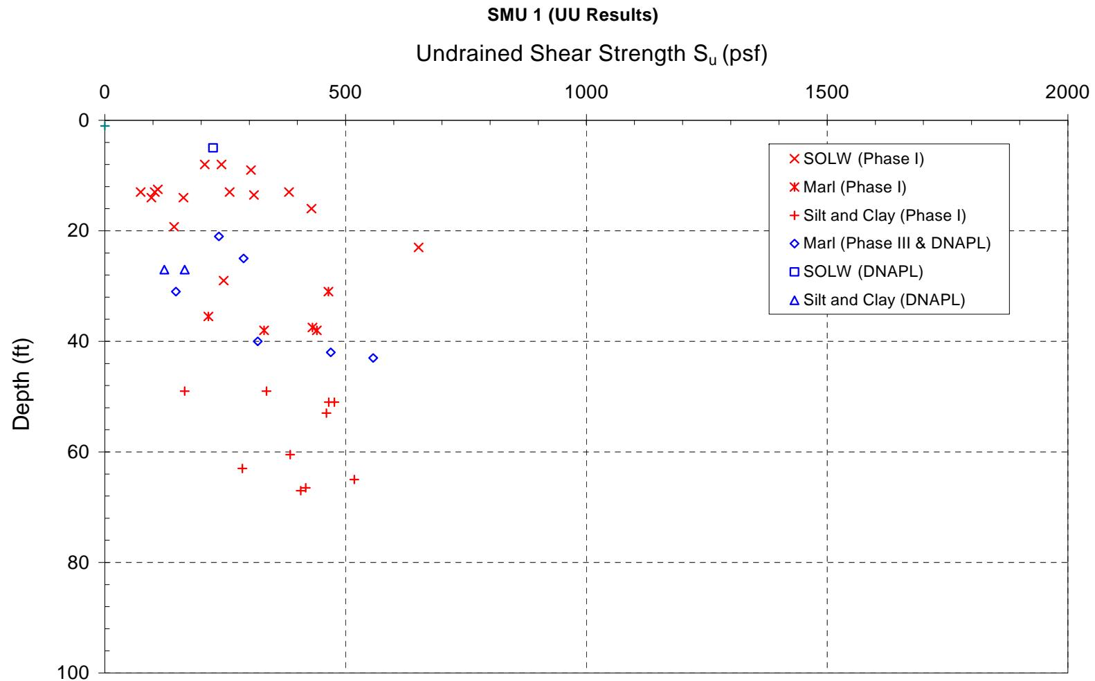
Figure 21. Undrained shear strength from UU tests
