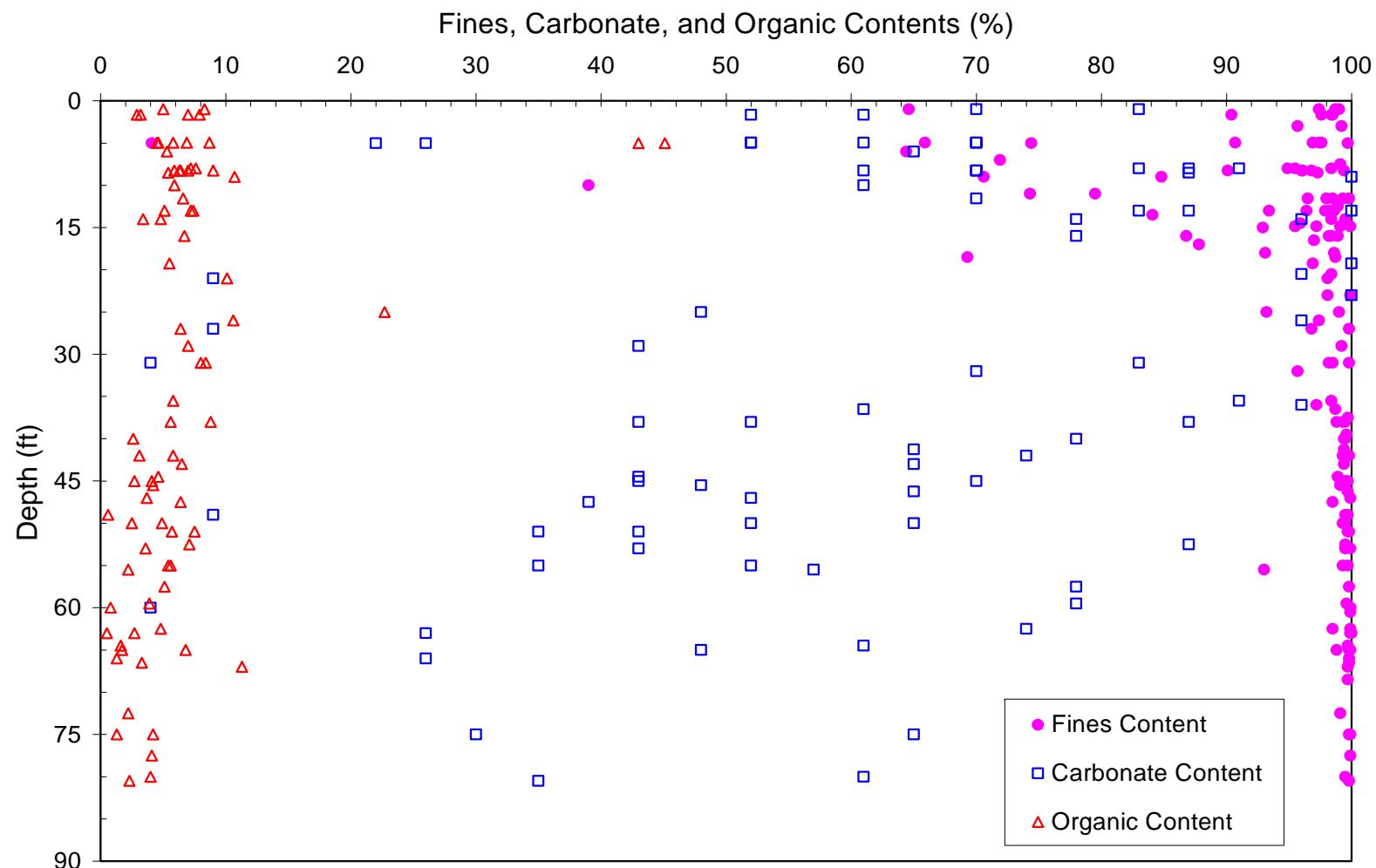
Figure 12. Plot of fines, carbonate, and organic contents versus depth
