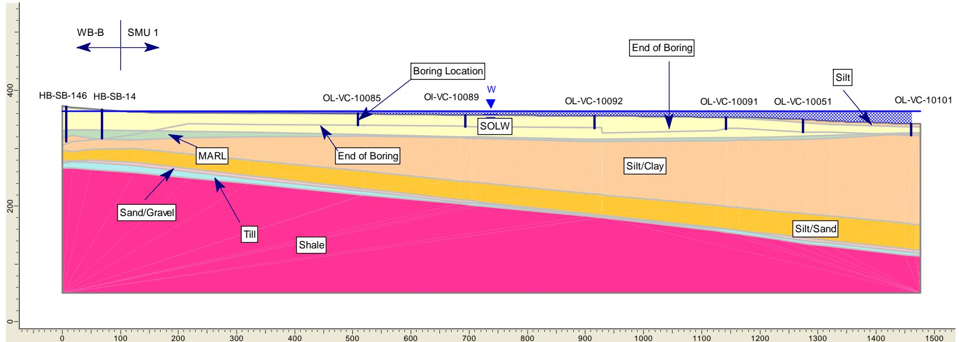
Figure 6. Geometry of cross section 4
