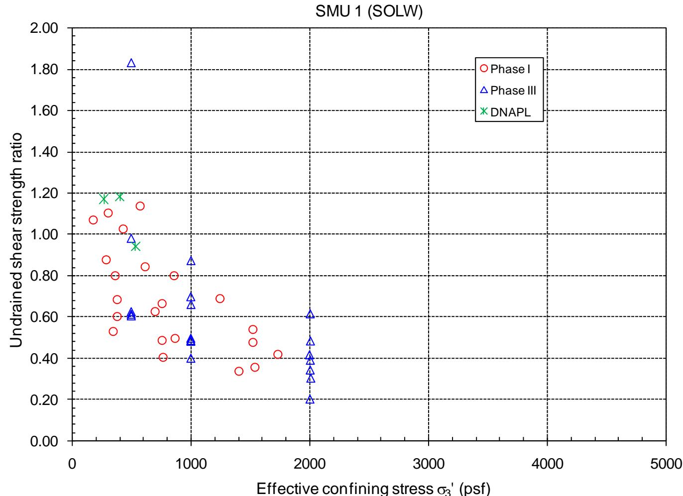
Figure 23. Undrained shear strength ratio for SOLW from CU tests
