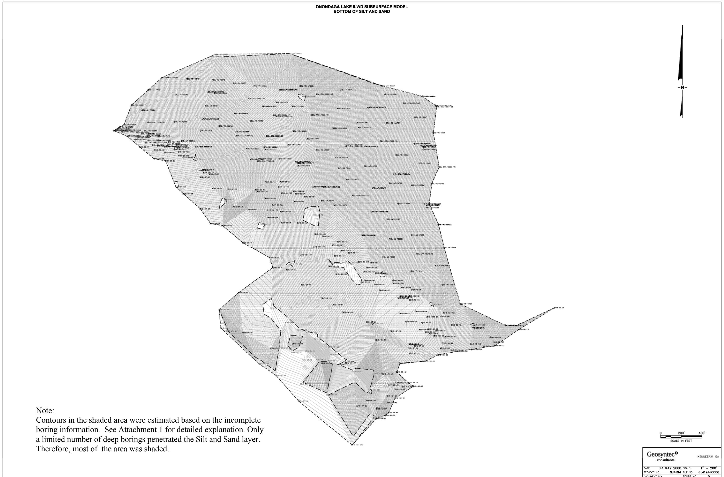
Figure 1-6. Contours of bottom of Silt and Sand
