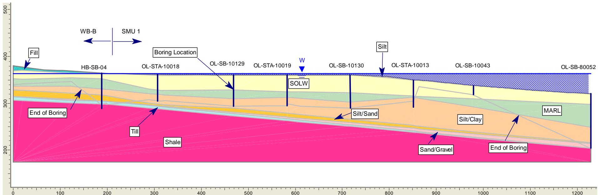
Figure 3. Geometry of cross section 1
