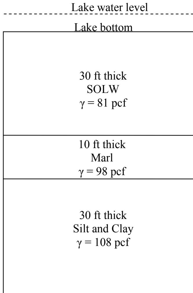
Figure 19. Assumed representative subsurface profile in the ILWD area
