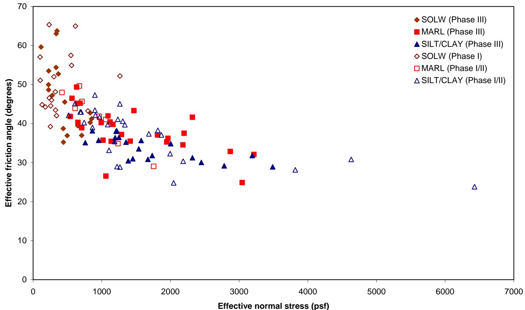
Figure 30. Effective stress friction angle versus effective normal stress for SOLW, Marl, and Silt and Clay
