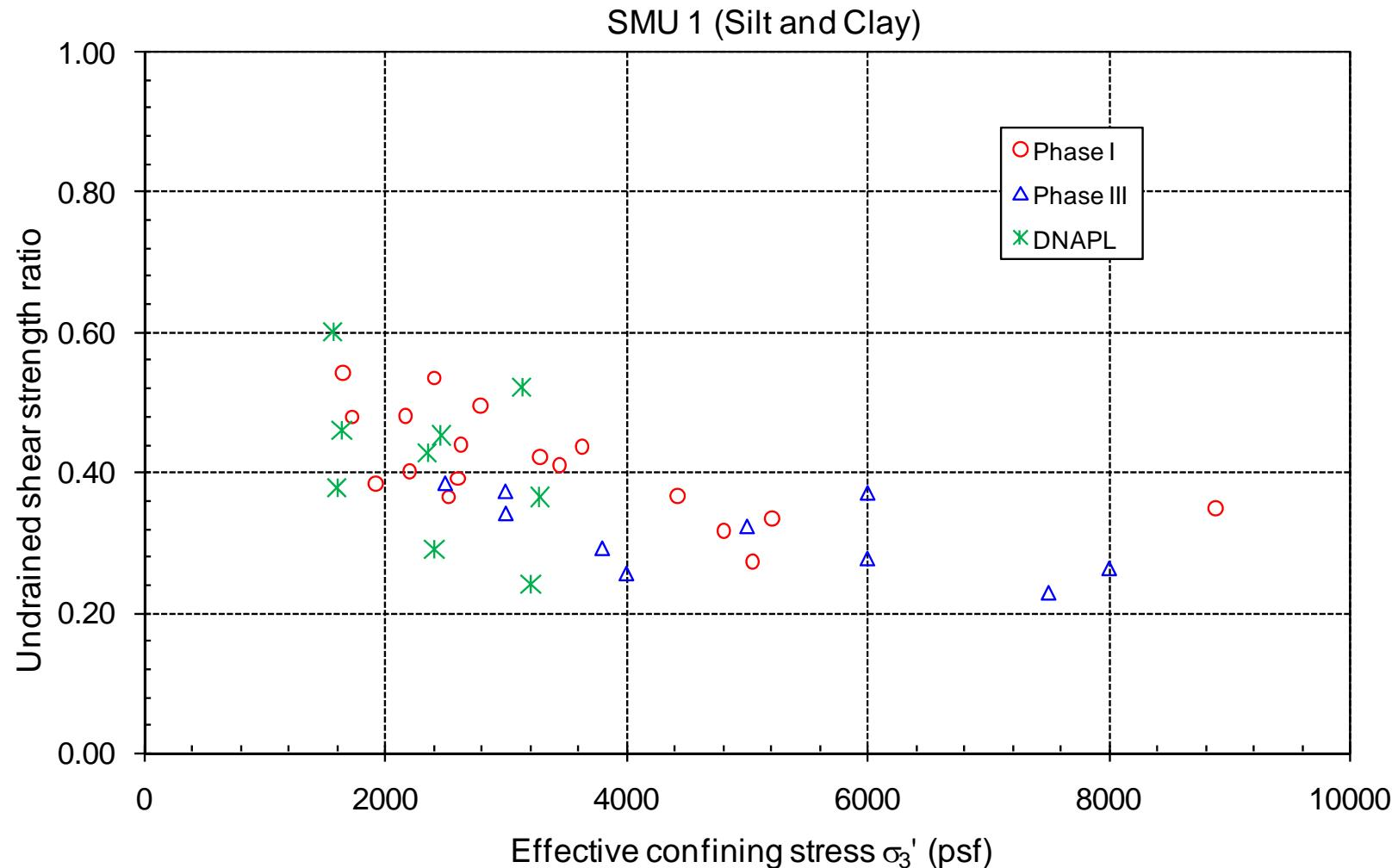
Figure 25. Undrained shear strength ratio for Silt and Clay from CU tests
