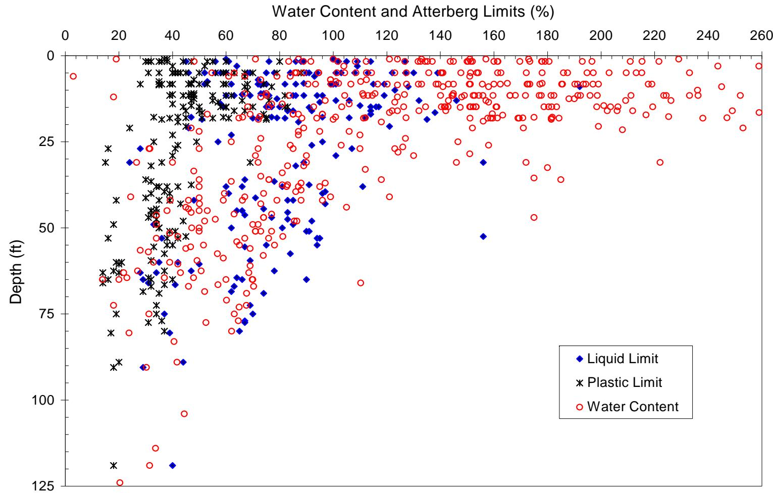
Figure 13. Plot of water content and Atterberg limits versus depth
