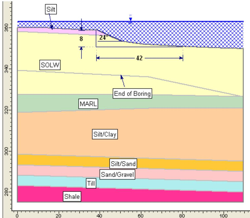
Figure 9. Geometry of cross section 7
