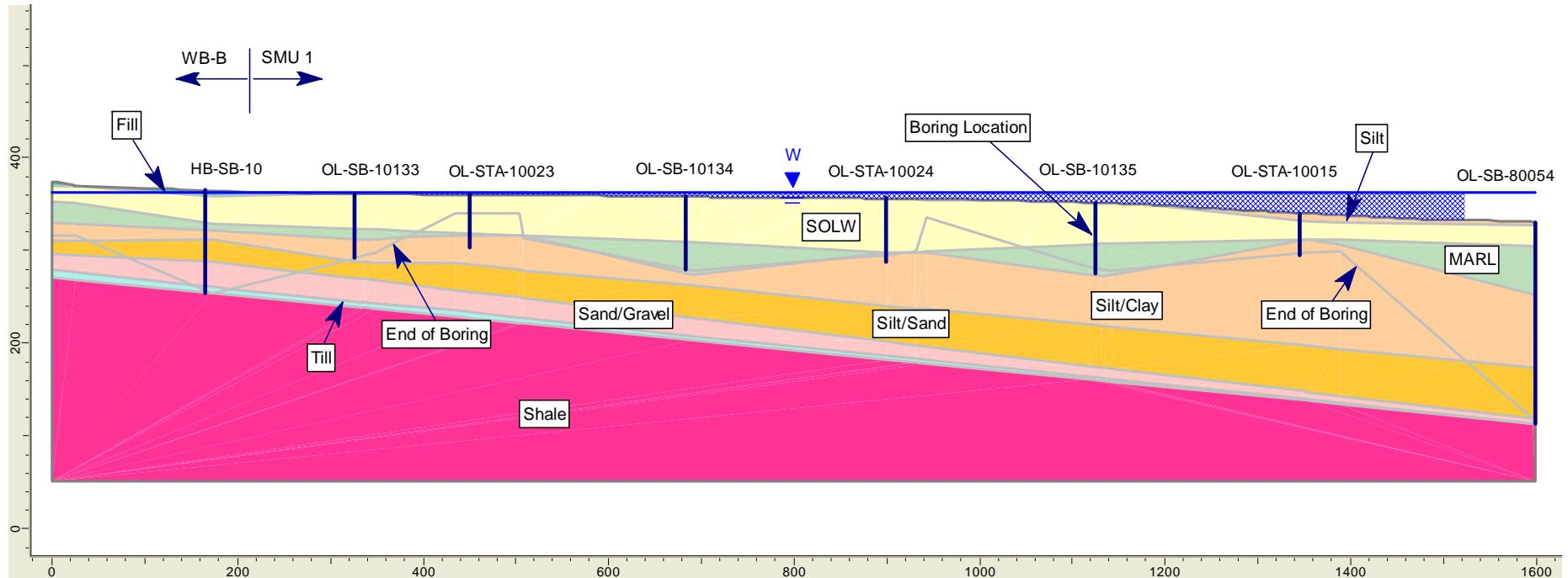
Figure 5. Geometry of cross section 3
