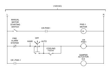
NOTE: PROVIDE AN 8"X6"X6" DEEP (MINIMUM) NEMA 4 SURFACE MOUNTED ENCLOSURE FOR PWE-1 HOA AND CONTROL RELAY CR-PWE1.
