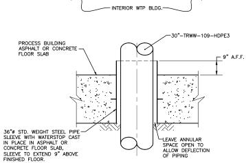
30" EFFLUENT-FLOOR PENETRATION DETAIL
