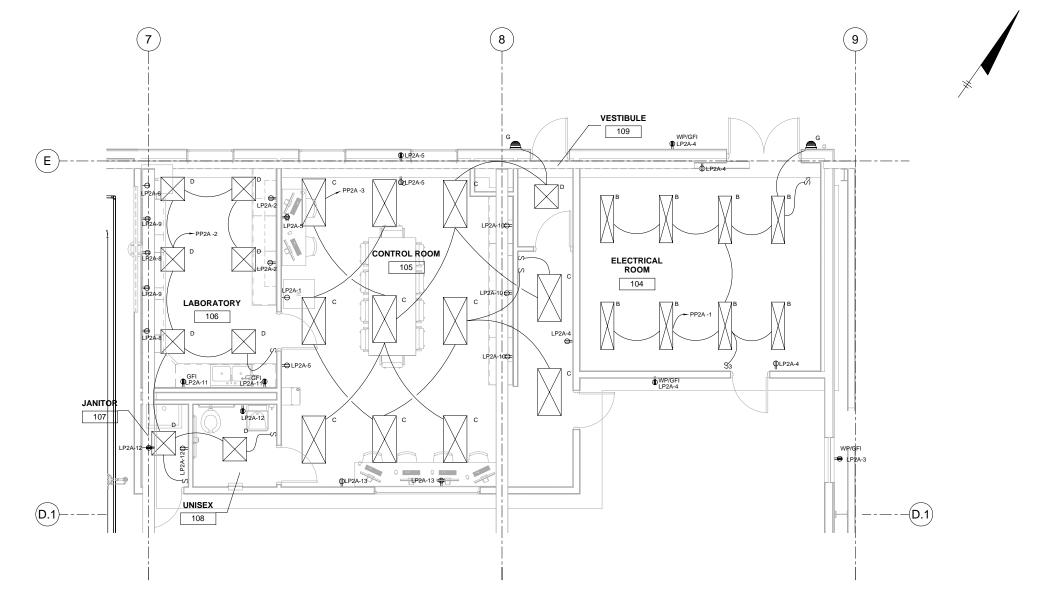
ENLARGED ELECTRICAL RM. 104/CONTROL RM. AREA LIGHTING PLAN SCALE: 1/4" = 1'-0"
