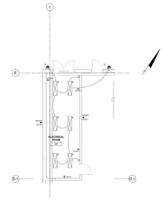
ELECTRICAL ROOM 101 ENLARGED LIGHTING PLAN SCALE: 1/4" = 1'-0"
