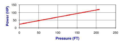
Design Point: 0 PSI Suction 96 FT Discharge 96 FT Diff. Pressure 1,653 GPM 1 CP
