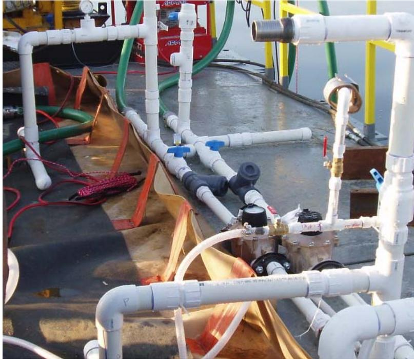
Raw water strainers, flow meters, and calibration riser.
