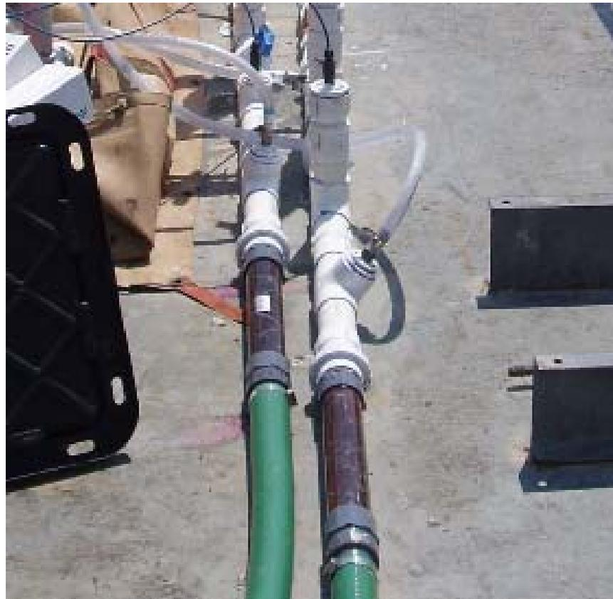
1:1 solution lines upstream of static mixers and the static mixers.
