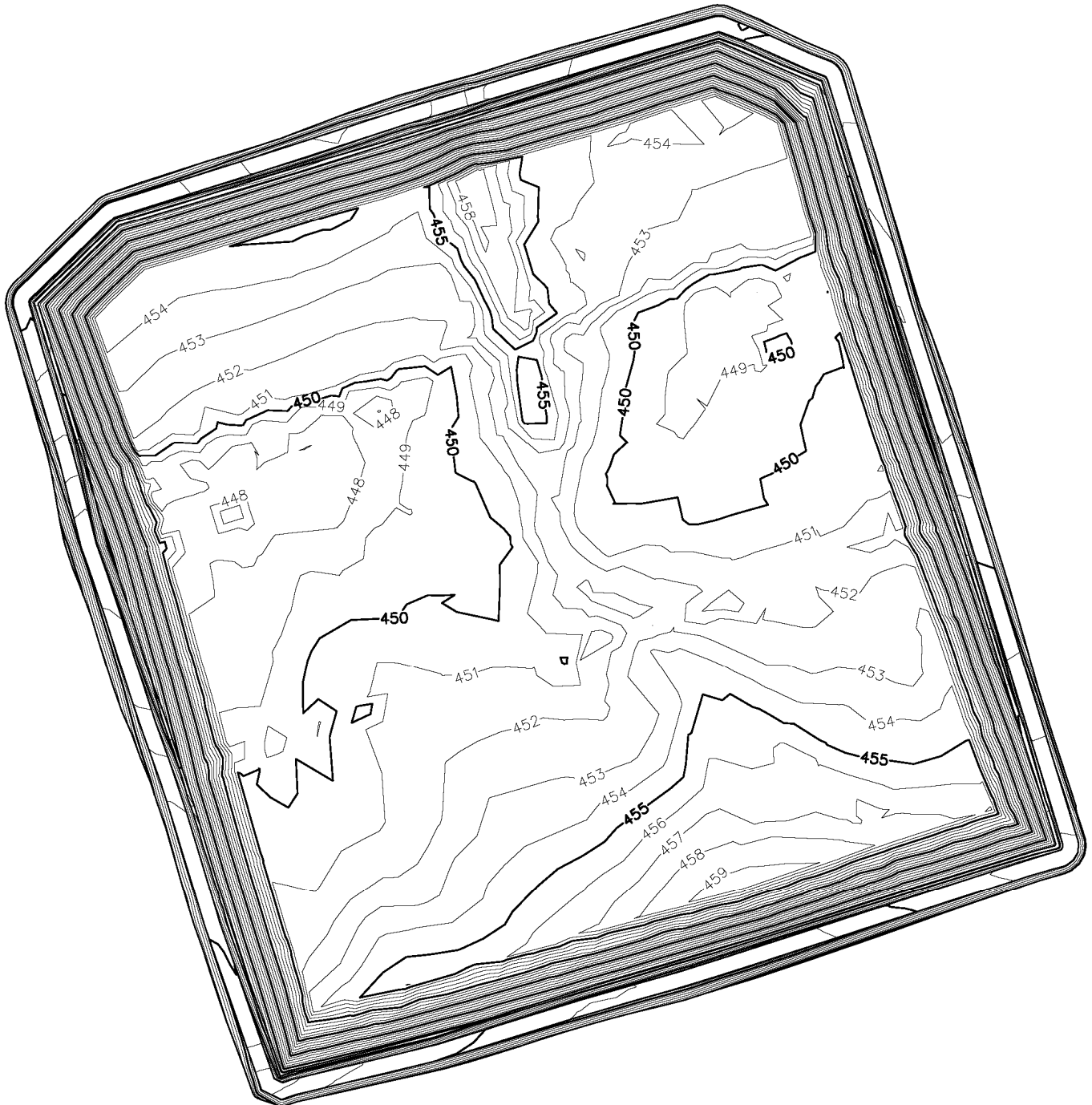
Figure 15. CASE 2: Top of Dredge Material in Geo-tubes Post-Settlement Elevation at the End of Year 4
