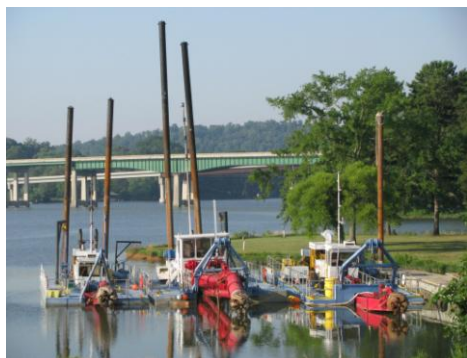
Hydraulic dredges similar to the dredges to be used at Onondaga Lake.
