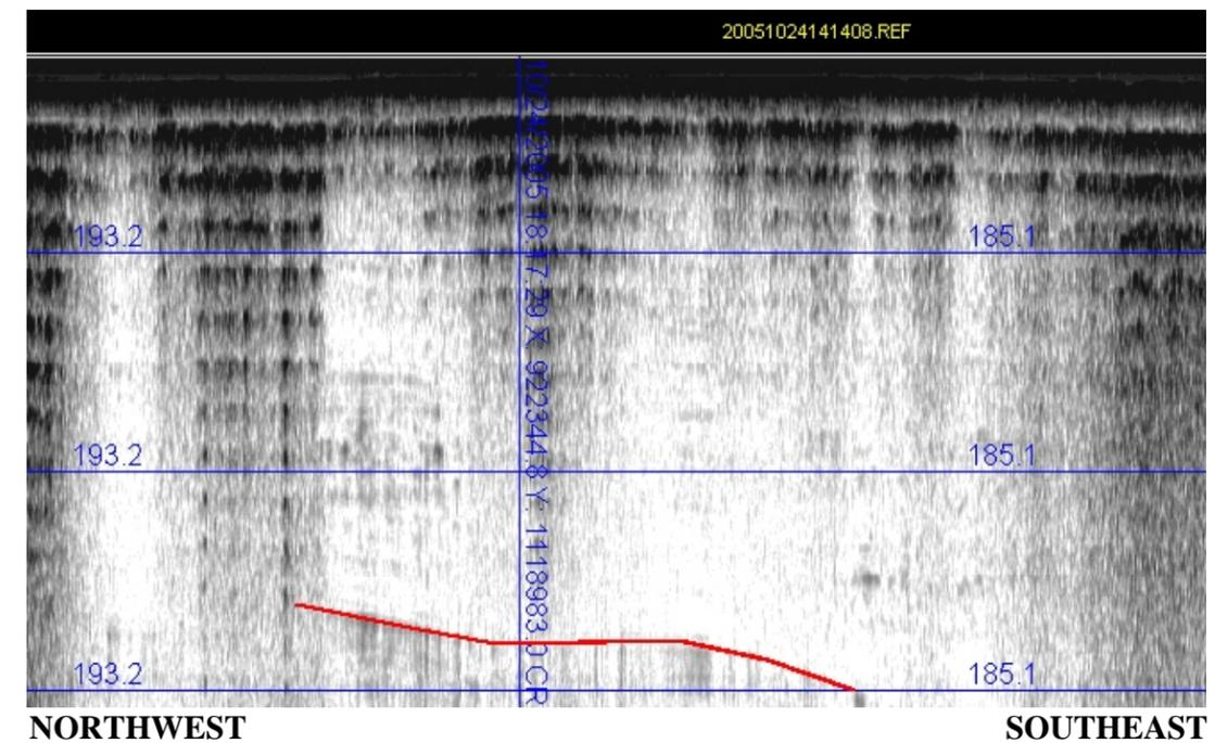
**PROFILE 2 - FILE 20051024141408-060-A:** 155 foot long segment of sub-bottom record suggests 50 feet of overburden material
