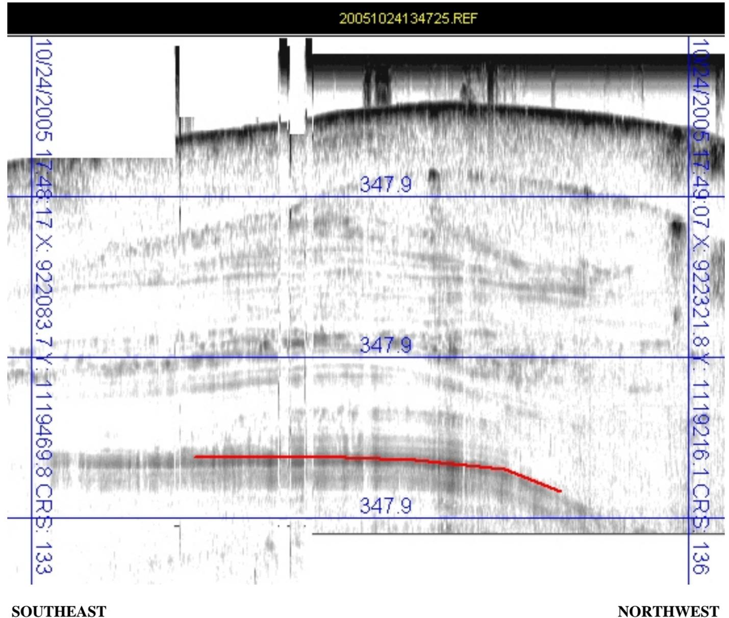
**PROFILE 4 - FILE 20051024134725:** 180 foot long segment of sub-bottom record suggests 44 feet of stratified overburden material.
