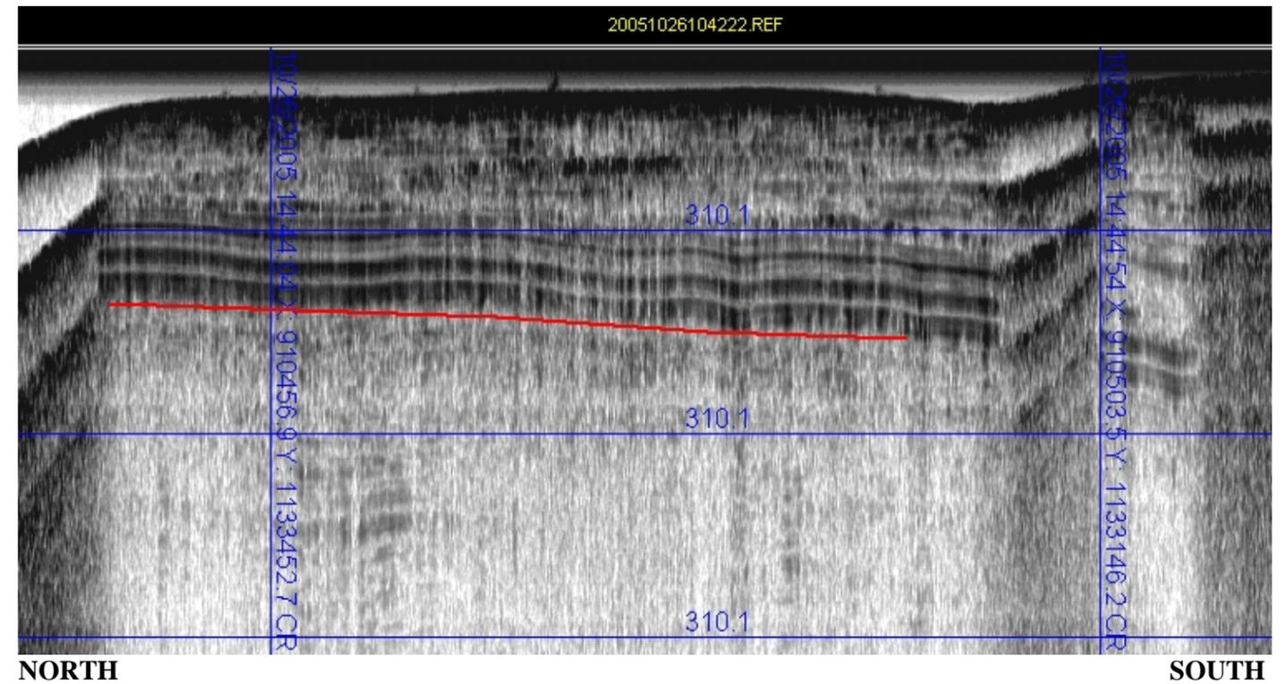
**PROFILE 2 - FILE 20051026104222:** 305 foot long segment of sub-bottom record suggests 19-23 feet of layered overburden material
