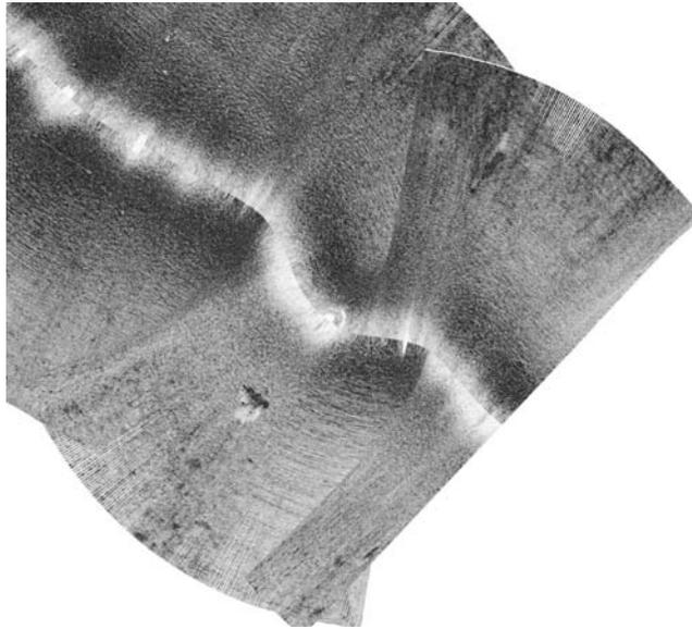
Same data as above, georeferenced using a short period smoothing algorithm. Contact "A" still masked by improperly projected pings due to its position relative to the start of the file.
