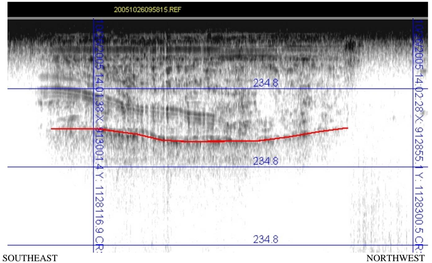
**PROFILE 1 - FILE 20051026095815:** 205 foot long segment of sub-bottom record suggests 29 feet of layered overburden material
