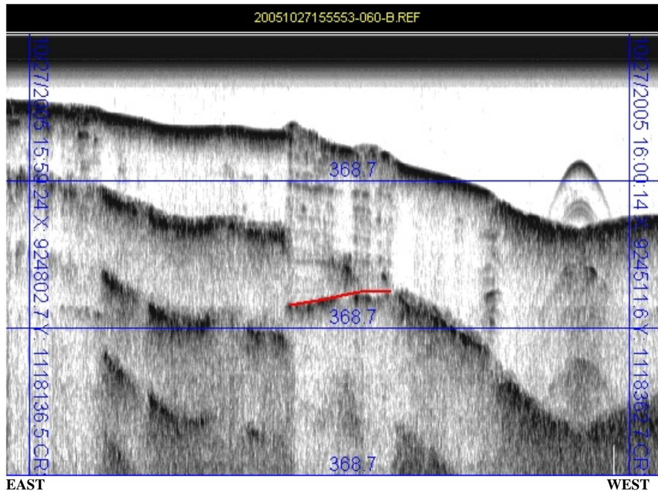
**PROFILE 3 - FILE 20051027155553-060-B:** 300 foot long segment of sub-bottom record. Penetration of 25 feet was achieved for a 70 linear foot portion. Outfall shown as parabolic reflector to right (west).
