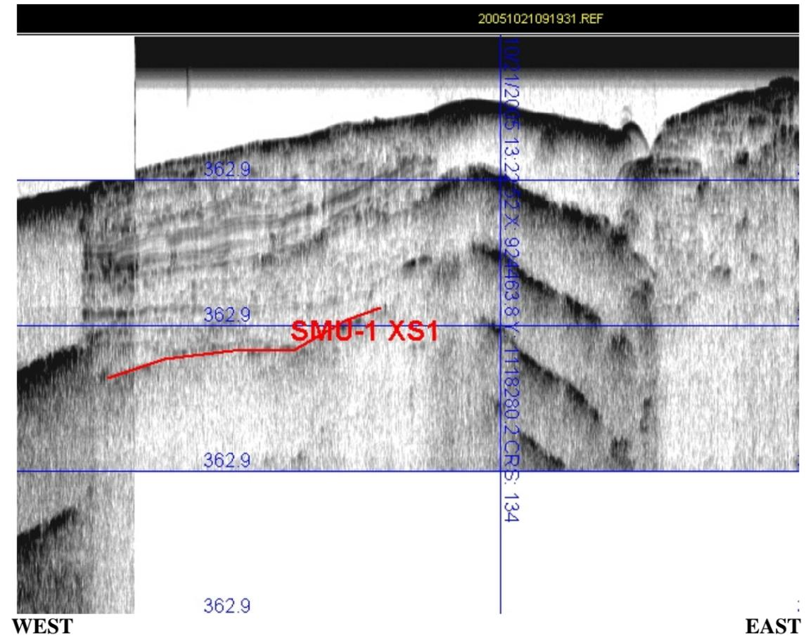
**PROFILE 1 - FILE 20051021091931:** 170 foot long segment of sub-bottom record depicting 27 feet of stratified material
