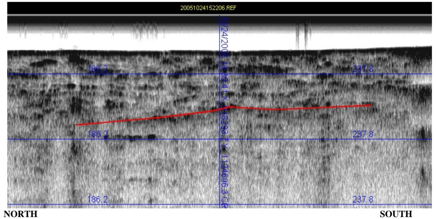
**PROFILE 1 - FILE 20051024152206:** 240 foot long segment of sub-bottom record *suggests* 17-23 feet of layered overburden material
