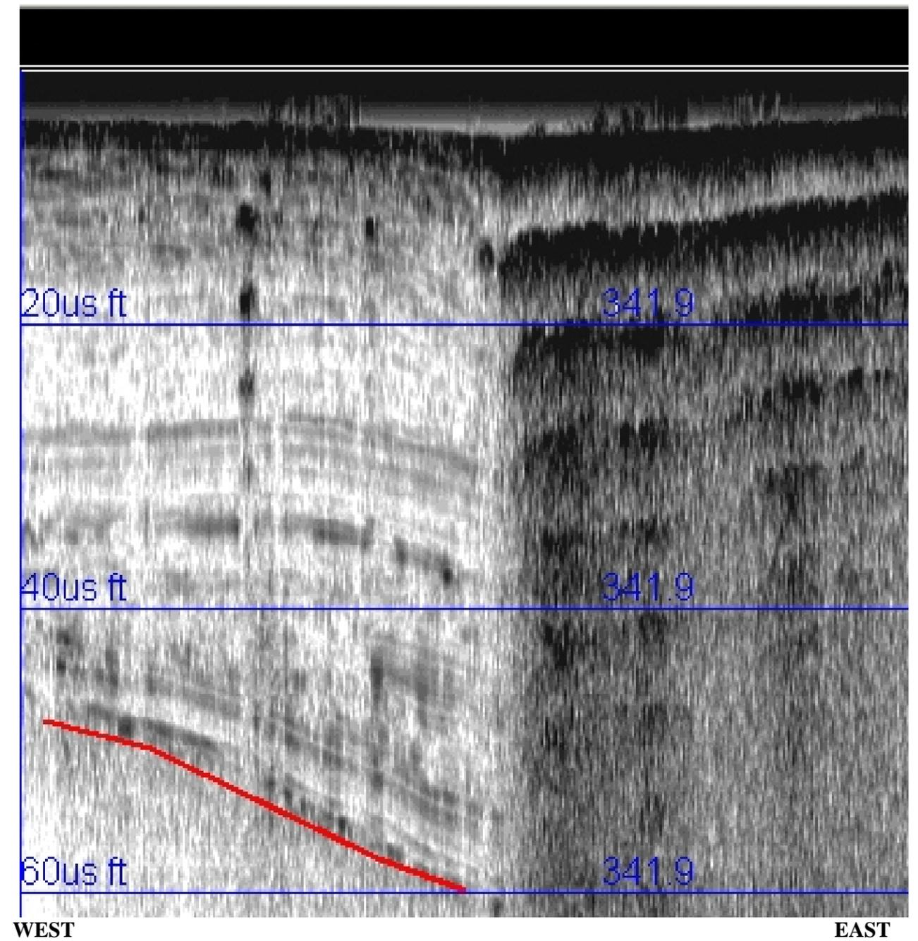
**PROFILE 3 - FILE 20051026155712:** 115 foot long segment of sub-bottom record suggests as much as 60 feet of stratified overburden material. The right hand side of the record depicts typical data for SMU4, with negligible penetration and strong multiple returns
