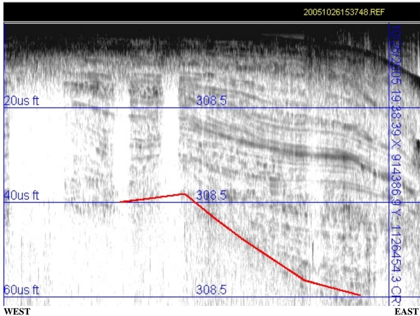
**PROFILE 2 - FILE 20051026153748:** 205 foot long segment of sub-bottom record *suggests* 35-52 feet of layered overburden material
