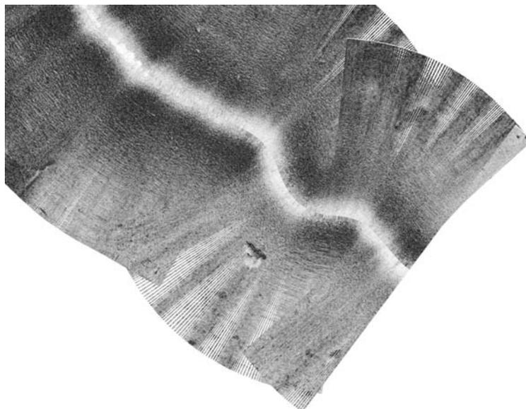
Same data as above, projected into real-space coordinates (i.e., georeferenced). Vessel track used as navigation, using an incorrect assumption that towfish yaw mimics vessel heading. Note that the large Contact “A” is masked by improperly projected data.
