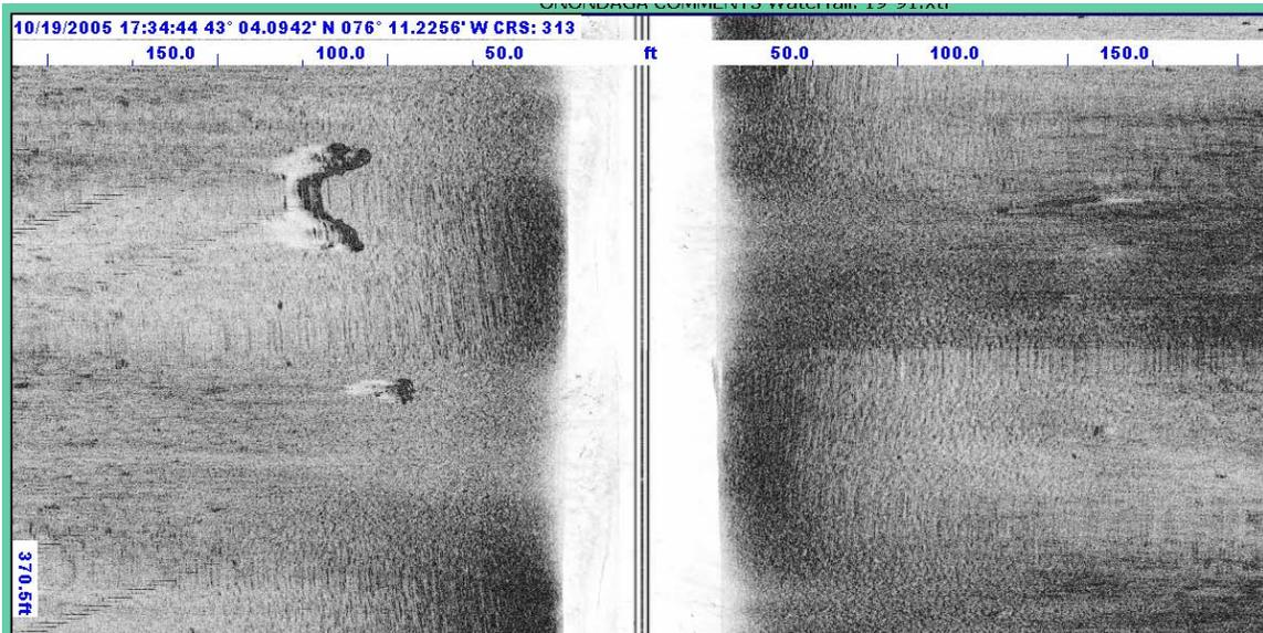
Raw data from sonar file 19-91.xtf depicts large objects (Contacts or Targets “A” and “B”) on port (left) channel, smaller targets on starboard channel. The vessel’s heading was roughly northwest and the beginning of the recording is the upper portion off the record. Note that Contact “A” is observed almost immediately after beginning the recording (~120 pings or 8 seconds).
