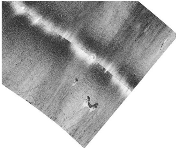
Same data as above, georeferenced using an extremely long period smoothing algorithm. Contact "B" and starboard Contacts visible, but towfish yaw is completely (and likely inappropriately) masked by navigation smoothing.
