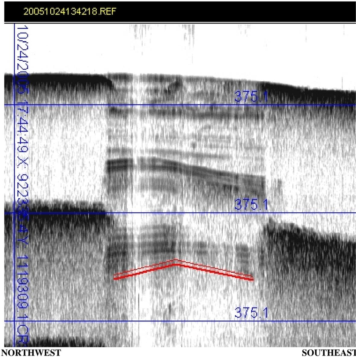
**PROFILE 3 - FILE 20051024134218:** 145 foot long segment of sub-bottom record suggests 37 feet of stratified overburden material.
