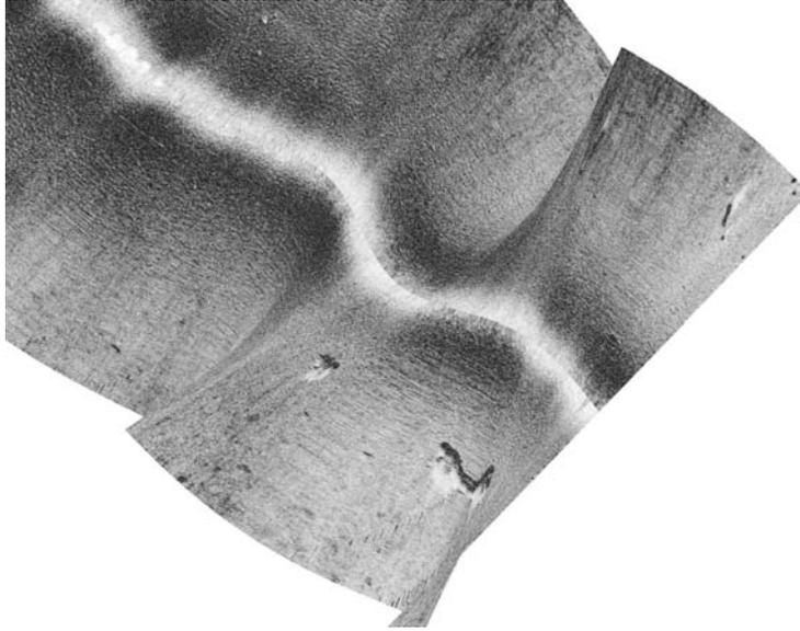
Same data as above, georeferenced using a longer period smoothing algorithm. Contact "B" and starboard Contacts visible as yaw period experienced by the towfish is approached.
