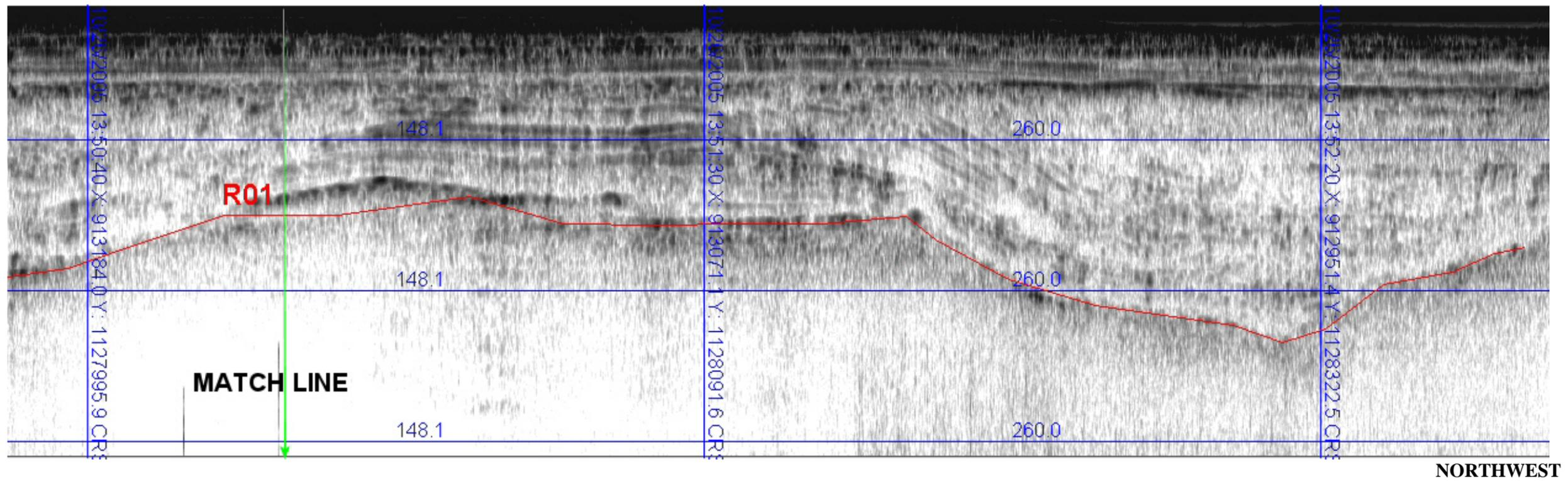
**PROFILE 2 - FILE 20051026094900-060-A:** 1,065 foot long segment of sub-bottom record suggests 29-42 feet of layered overburden material
