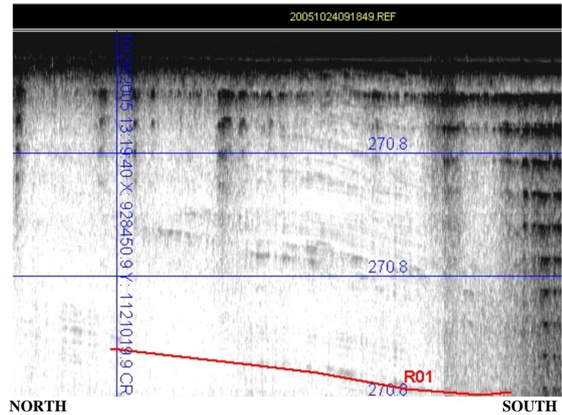
**PROFILE 1 - FILE 20051024091849:** 270 foot long segment of sub-bottom record suggests 46-54 feet of layered overburden material (note the abrupt loss of penetration at the right (southern) portion of the record)
