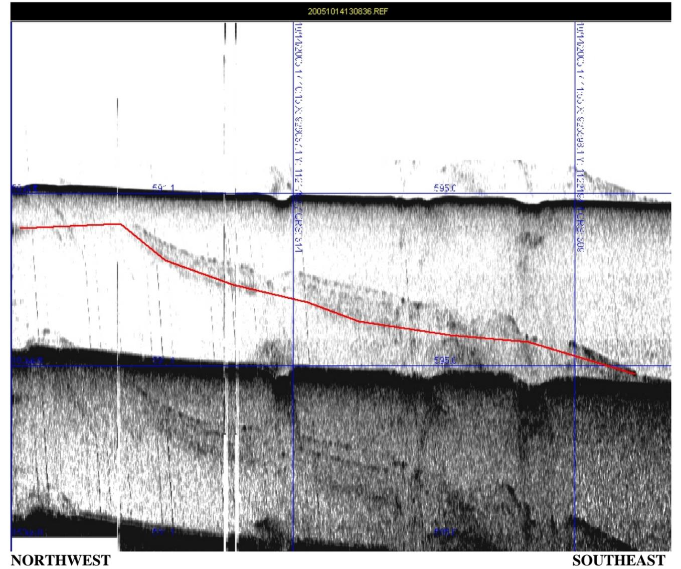
**PROFILE 3 - FILE 20051014130836-120-A:** This 1,300 foot long portion of sub-bottom sonar record suggests up to 50 feet of sediment and depicts three anomalous depressions. The indicated reflector is suspect due to potential multipath interference. The depths of the depressions are approximately 2.5 – 3 feet and widths are approximately 60 – 80 feet. Turbulence is present in the water column directly above one of the depressions.
