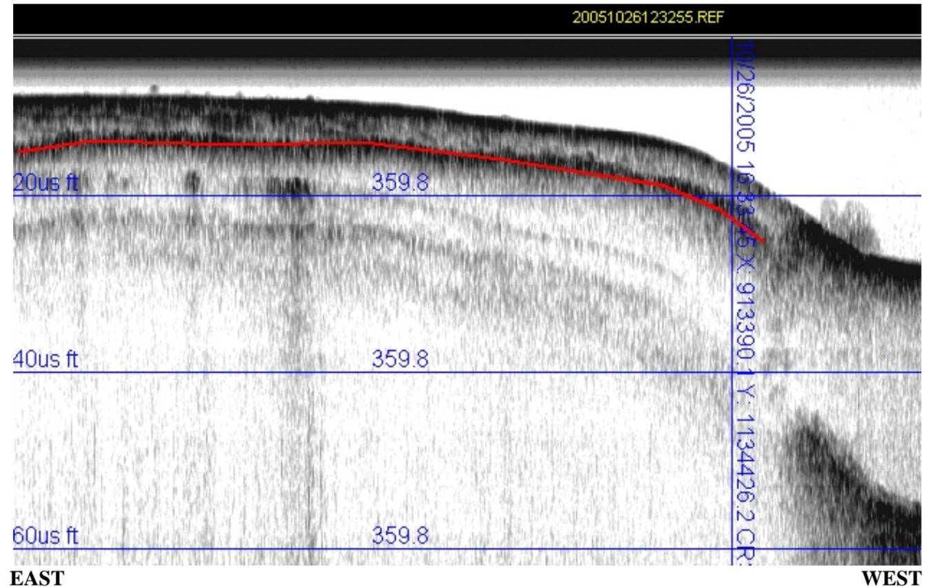
**PROFILE 1 - FILE 20051026123255:** 425 foot long segment of sub-bottom record suggests 7-9 feet of overburden material
