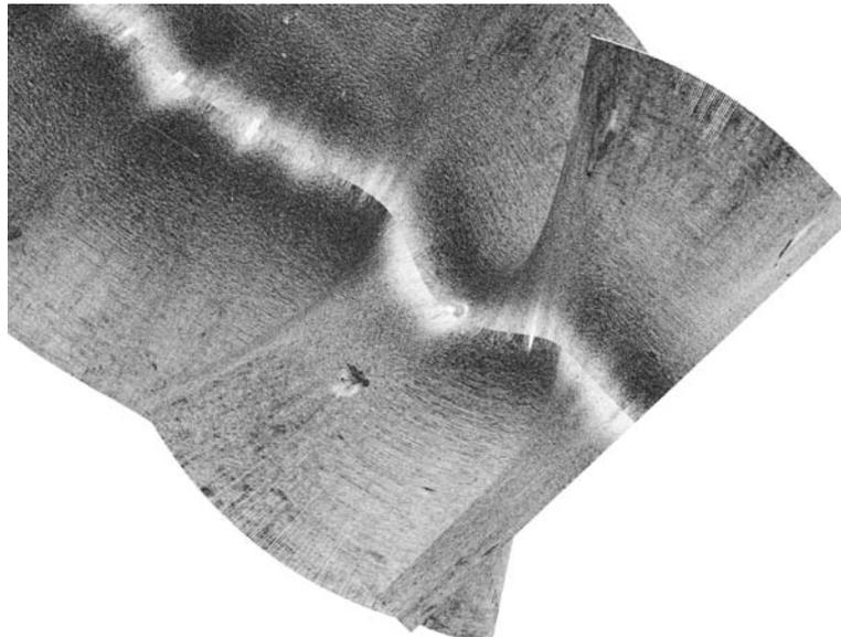
Same data as above, georeferenced using a longer period smoothing algorithm. Contact "A" still masked by improperly projected pings due to its position relative to the start of the file.
