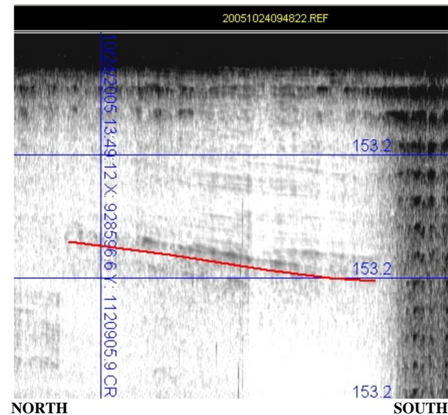
**PROFILE 2 - FILE 20051024094822:** 80 foot long segment of sub-bottom record suggests 31-37 feet of layered overburden material (note the abrupt loss of penetration at the right (southern) portion of the record)
