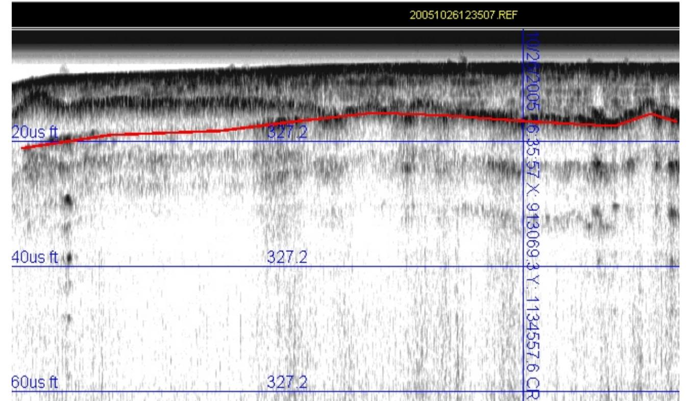
**PROFILE 2 - FILE 20051026123507:** 375 foot long segment of sub-bottom record suggests 5-7 feet of overburden material
