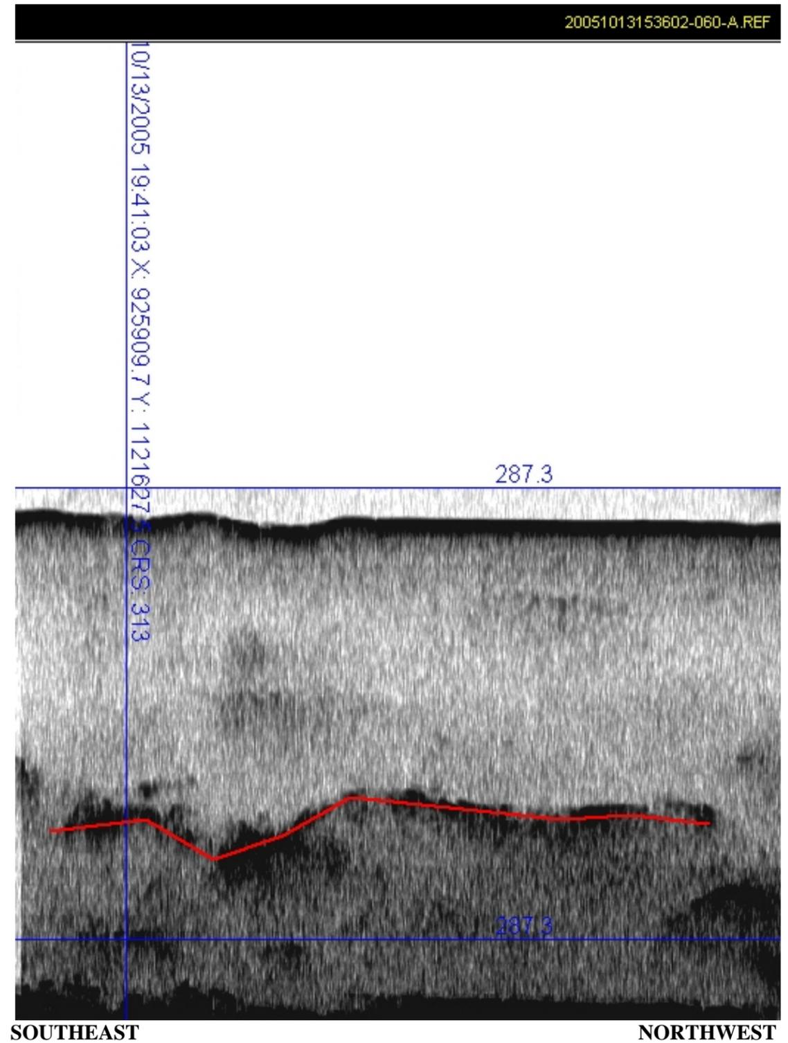
**PROFILE 1 - FILE 20051013153602-060-A:** 260 foot long segment of sub-bottom record *suggests* at least 37 feet of overburden material
