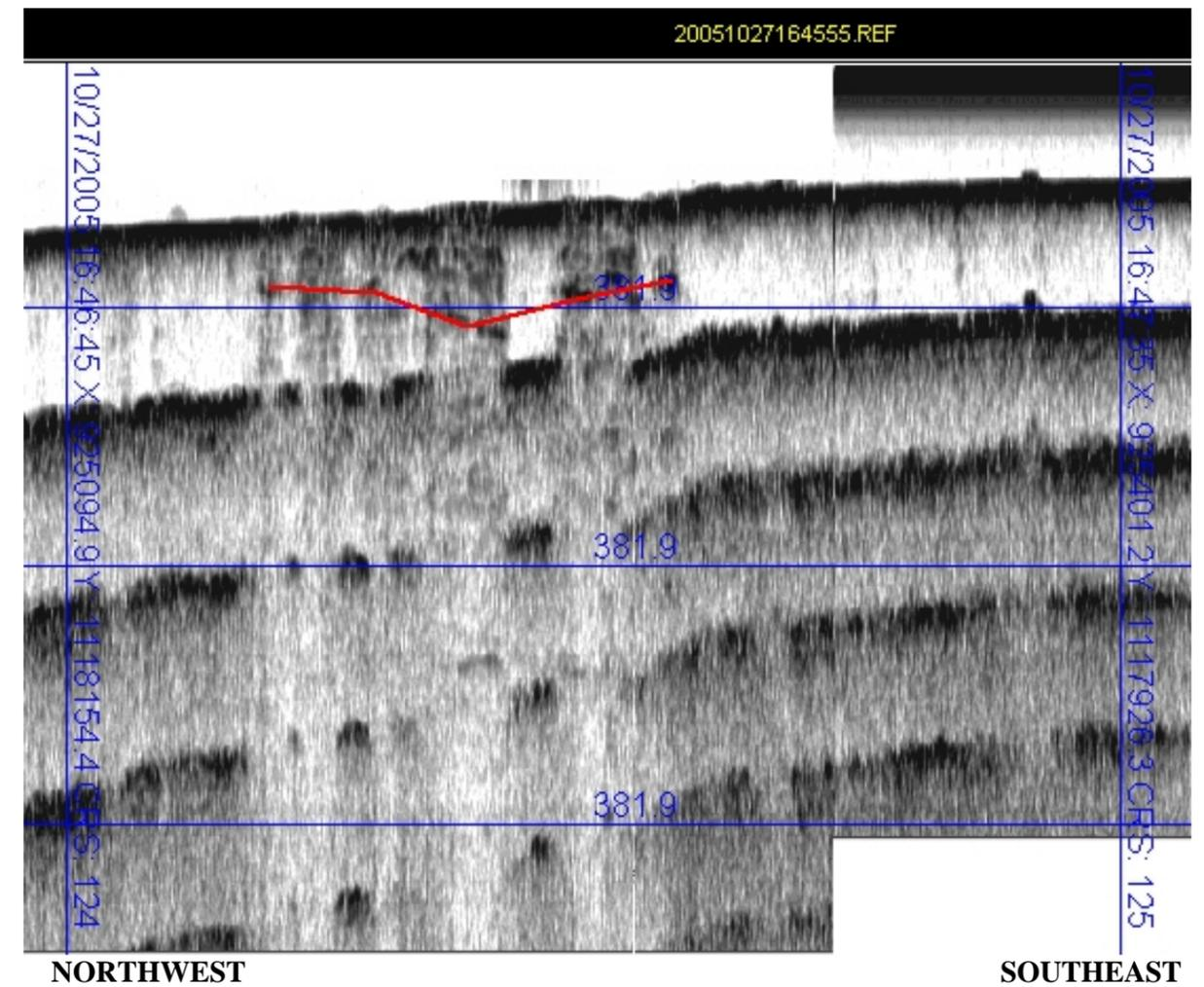
**PROFILE 4 - FILE 20051027164555:** 145 foot long segment of sub-bottom record depicting 6-10 feet of stratified material
