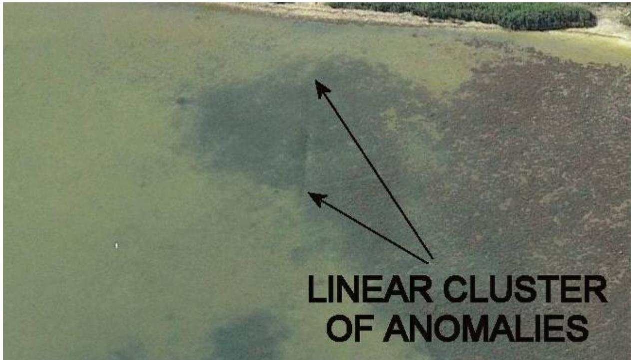
**Photograph 4.** *Close-up of an aerial photograph (looking south) which identifies the same linear bottom feature approximately co-located with a linear arrangement of magnetic anomalies.*
