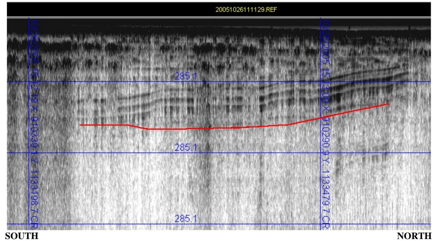
**PROFILE 1 - FILE 20051026111129:** 310 foot long segment of sub-bottom record suggests 26-32 feet of layered overburden material
