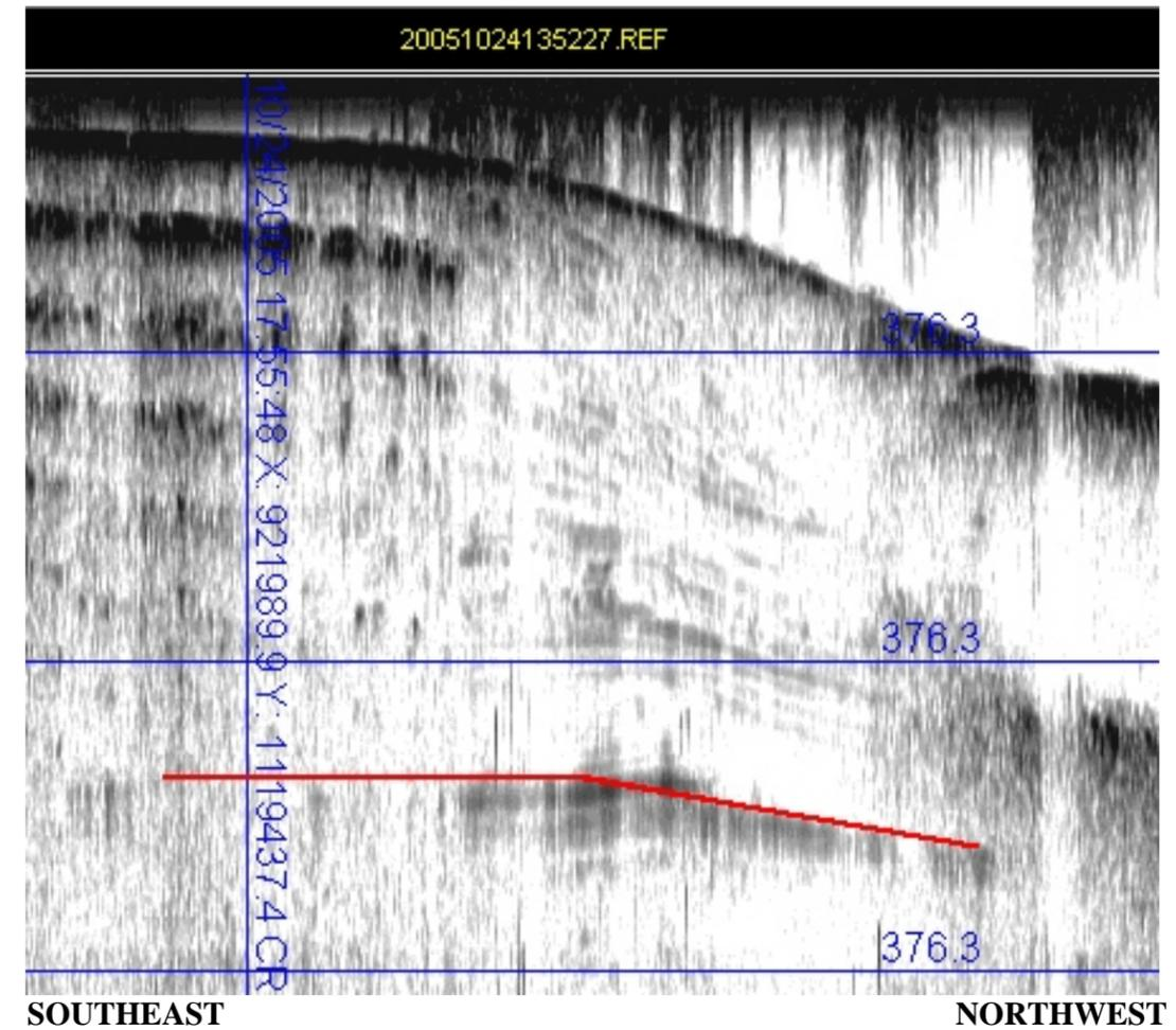
**PROFILE 1- FILE 20051024135227:** 240 foot long segment of sub-bottom record suggests 40 feet of overburden material
