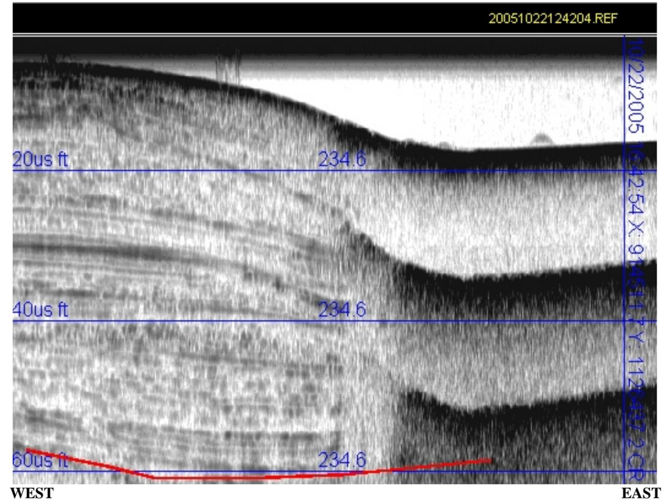
**PROFILE 1 - FILE 20051022124204:** 195 foot long segment of sub-bottom record *suggests* 55-60 feet of layered overburden material.
