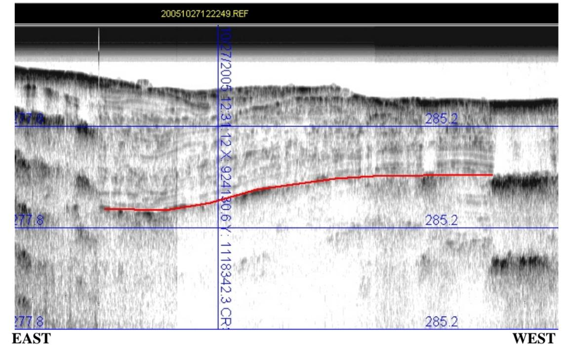
**PROFILE 2 - FILE 20051027122249:** 300 foot long segment of sub-bottom record depicting 15-5 feet of stratified material
