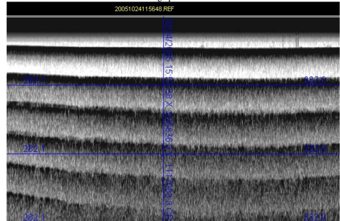
**PROFILE 2 - FILE 20051024115648:** Typical sub-bottom record for SMU 7. The sonar signal did not penetrate the sediment. The record above depicts the sediment surface and five multiple returns.
