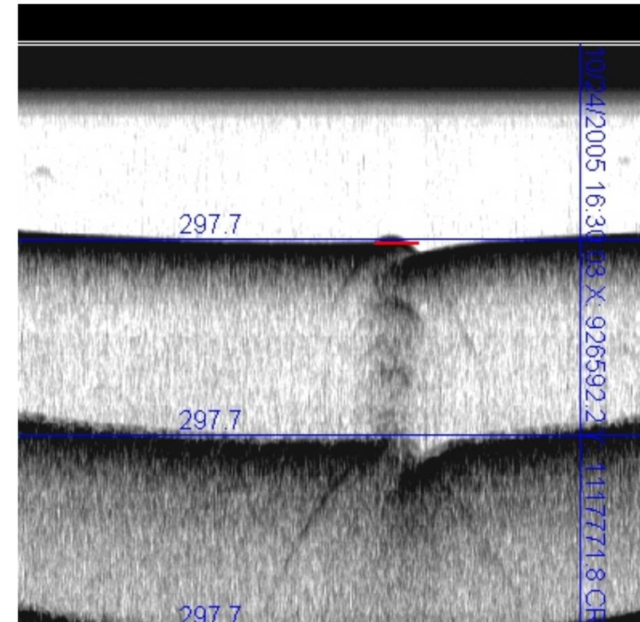
**PROFILE 1 - FILE 20051024122823:** Large parabolic reflector indicates outfall
