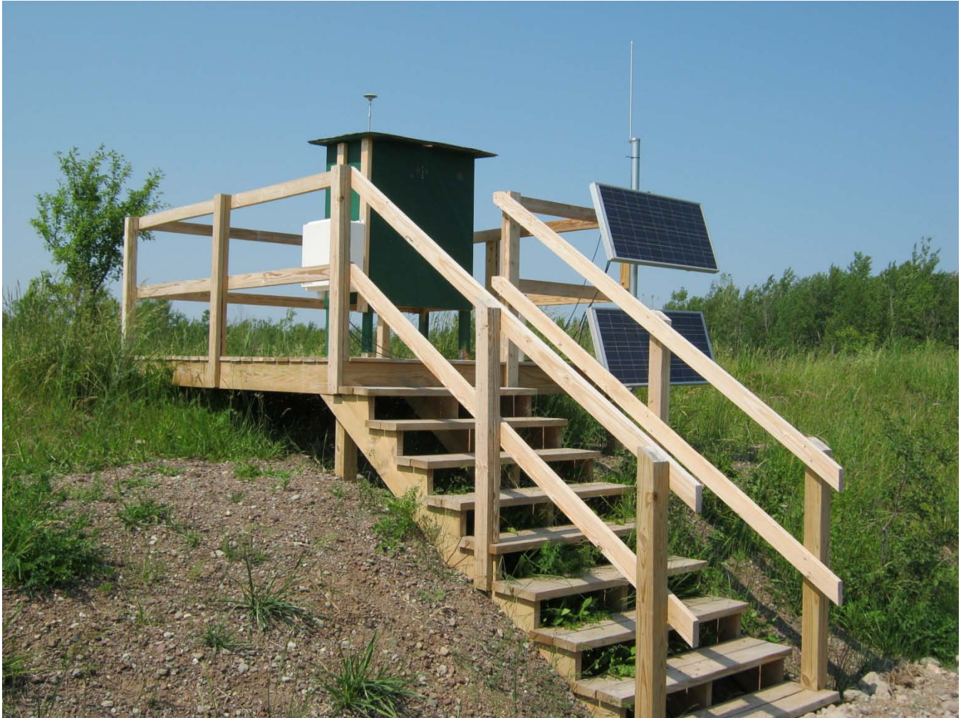
Figure 5.3-2 Typical AQM Station – Showing Solar Panels, Weather-proof Data logger Enclosure, and ADR Omni-directional Inlet
