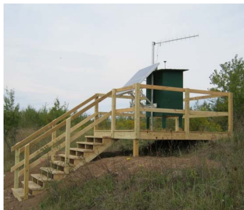
One of the eight air monitoring stations located at the sediment consolidation area site perimeter. See page 2 for the locations.
