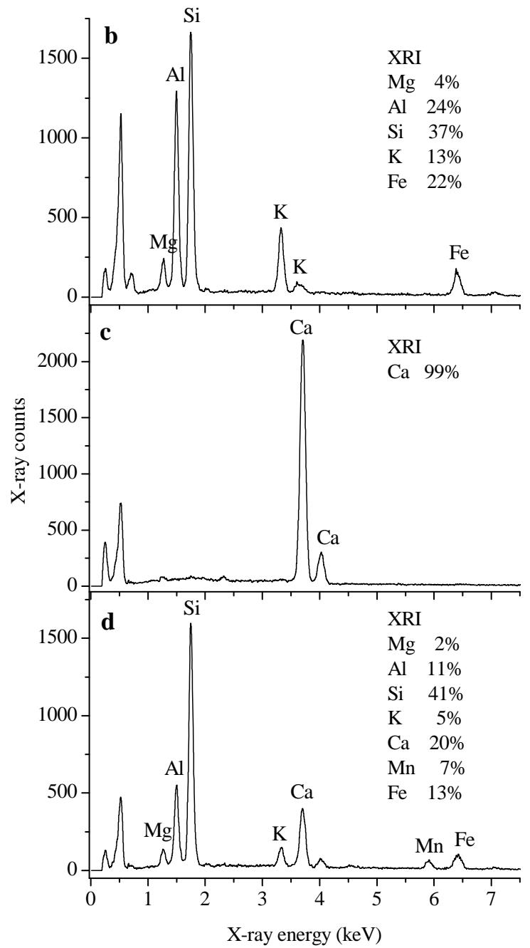
Fig. 4. Scanning electron micrographs of an aggregate from the 17 m trap sample collected on Oct. 22, 2012, along with X-ray spectra acquired from various points on the particle: (a) the large, compact aggregate; (b-d) X-ray spectra showing compositional signatures of ‘Clay’, ‘Calcite’, and ‘Ca-agg’, respectively.
