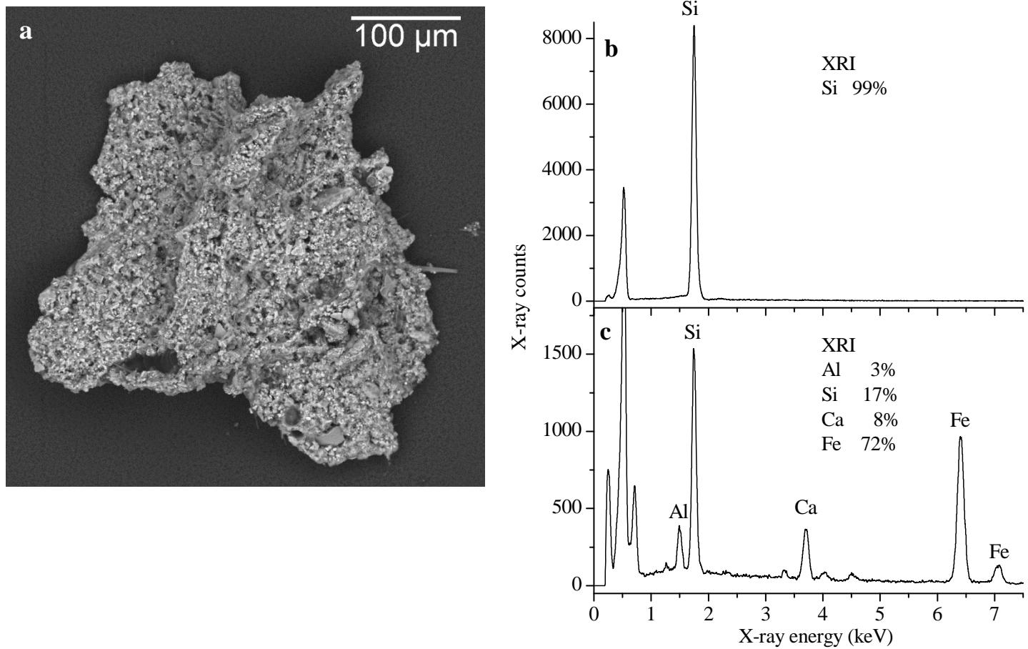
Fig. 3. Scanning electron micrographs of an aggregate (a) from the 17 m trap sample collected on Oct. 2, 2012, along with X-ray spectra from two different points of acquisition (b, c; typical of ‘Quartz’ and ‘Fe-rich’ particles, respectively). Relative X-ray intensities (XRI) of elements are listed in each spectrum.
