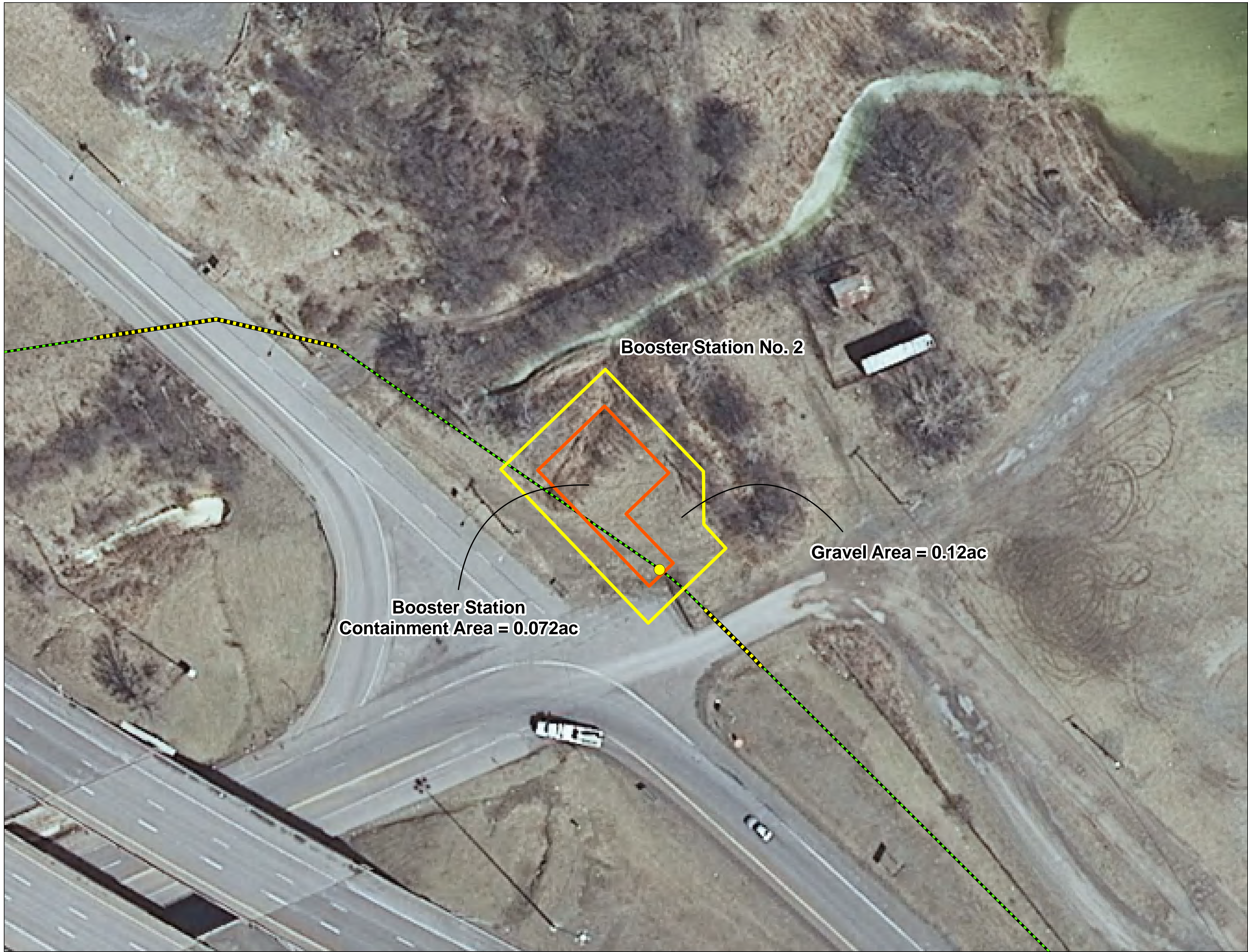
Figure 9 Booster Station No. 2 Layout Water Treatment Plant & Sediment Consolidation Area SWPPP PARSONS 301 Plainfield Road, Suite 350, Syracuse, NY 13212
