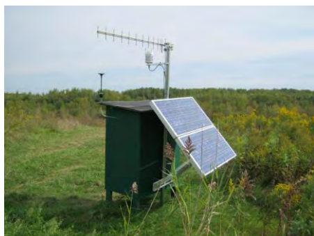
Air quality monitoring station being used for the Onondaga Lake project
