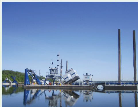
The largest of three hydraulic dredges (left) that will remove about 2 million cubic yards of material from the lake bottom. The cutter head (right) breaks up the lake bottom material before it is transferred into the pipeline.
