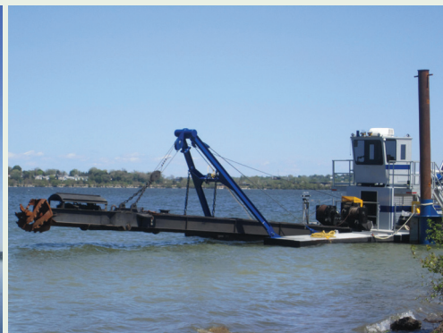
The largest of three hydraulic dredges (left) that will remove about 2 million cubic yards of material from the lake bottom. The cutter head (right) breaks up the lake bottom material before it is transferred into the pipeline.
